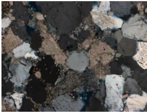
**Figure 7.4** Observed at 10x magnification. In XN, Subhedral quartz and slightly globular calcite that is interspersed between quartz grains acting as a cementing material.
