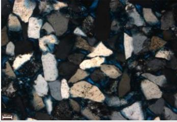
This image shows subhedral quartz grains, some intergrown. Pore space is also shown by blue epoxy. (10x, XN)
