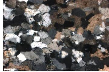
Quartz grains in this image are cemented by calcite. Some polycrystalline quartz is present as well. (10x, XN)
