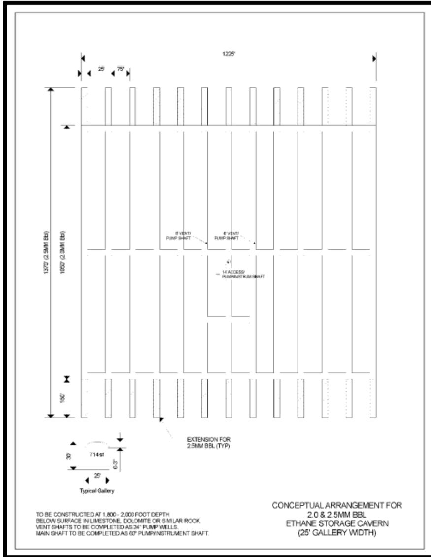
Figure 4. Plan view conceptual design for a mined-rock cavern (Nelson and others, 2011).
