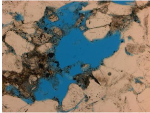
**Figure 11.10** Observed at 10x magnification. In PL, the blue dye represents the open pore spaces in the thin section, estimating about 11% porous overall.
