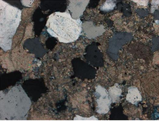
**Figure 4.7** Observed at 10x magnification. In XPL, deformed calcite grain and calcareous cement with subrounded, subhedral, undulose quartz grains. Some grains are slightly deformed from growth.
