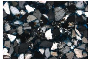
Two grains of plagioclase feldspar, sedimentary rock fragments, and subhedral quartz grains are shown in this image. (10x, XN)
