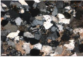
This image shows a subhedral grain of plagioclase feldspar. Sedimentary rock fragments, calcite grains, and intergrown quartz are also shown here. (10x, XN)
