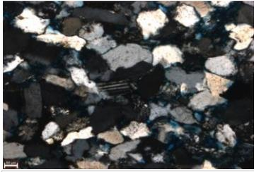
This image shows plagioclase feldspar with albite twinning surrounded by intergrown quartz grains.
