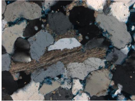
**Figure 5.2** Observed at 10x magnification. In XN, anhedral and slightly deformed undulose quartz with a elongated calcite grain deformed from quartz growth, acting as cementing material.
