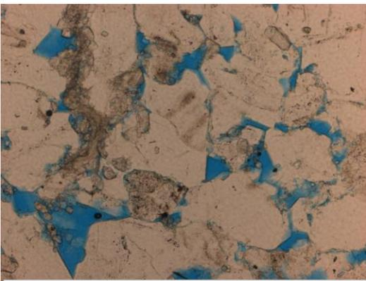
**Figure 4.11** Observed at 10x magnification. In PPL, the blue dye exhibits the open pore spaces in the thin section. Visual estimate of porosity is 13% porous.
