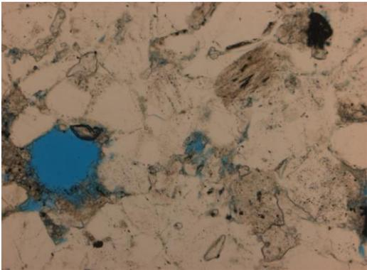
**Figure 8.9** Observed at 10x magnification. In PL, blue dye represents the open pore spaces in the thin section, estimating 5% porosity overall.
