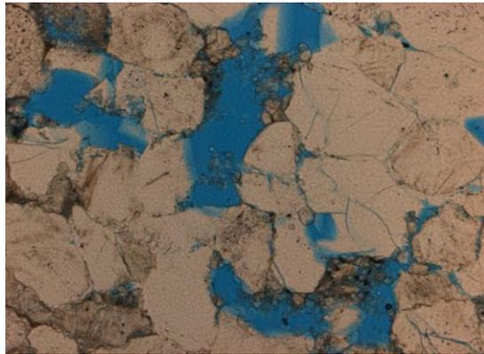
**Figure 6.8** Observed at 10x magnification. In PL, the blue dye indicates the open pores spaces in the thin section. This thin section has an estimated 9% porosity overall.
