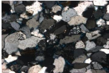
Sedimentary rock fragments are cemented in grains of intergrown quartz.
