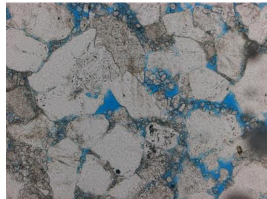
**Figure 5.12** Observed at 10x magnification. In PL, blue dye exhibits the open pore spaces in the thin section. The estimated porosity of the thin section is 11% overall
