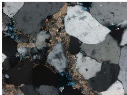
**Figure 9.6** Observed at 10x magnification. In XN, intergrown calcite cementing together subhedral undulose quartz. Also quartz overgrowth, cementing grains together.
