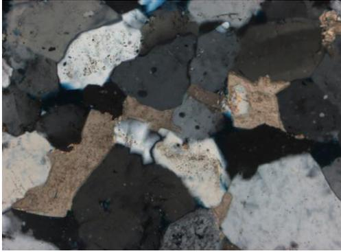
**Figure 9.7** Observed at 10x magnification. In XN, interspersed subhedral quartz and calcite grains. Both acting as cementing material.
