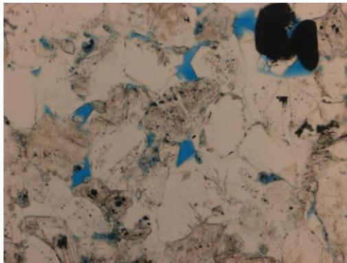
**Figure 7.10** Observed at 10x magnification. In PL, the blue dye represents the open spaces in the thin section, estimating to about 8% porosity overall.
