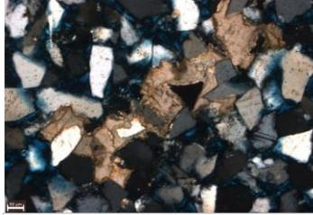
Subangular calcite cements quartz grains in this image. Blue epoxy shows pore space here as well. (10x, XN)
