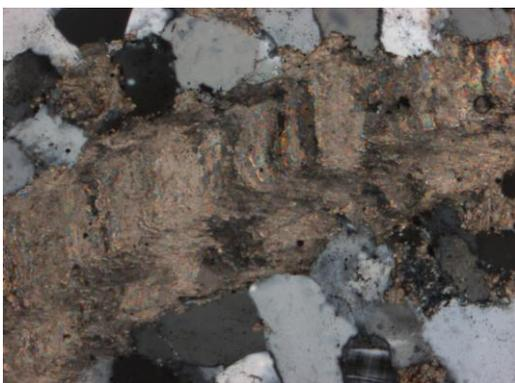
**Figure 8.5** Observed at 10x magnification. In XN, large, elongated, deformed calcite intergrown between subhedral quartz grains.
