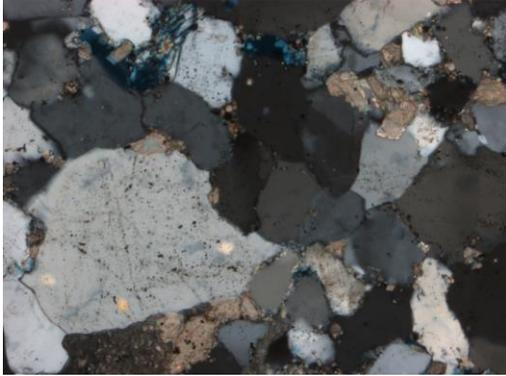
**Figure 7.7** Observed at 10x magnification. In XN, anhedral to subhedral quartz grains. some slight deformation from quartz growth.
