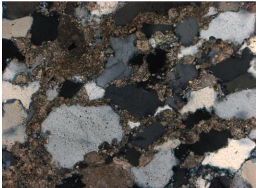
**Figure 5.5** Observed at 10x magnification. In XN, subhedral undulose quartz grains cemented together by deformed calcite
