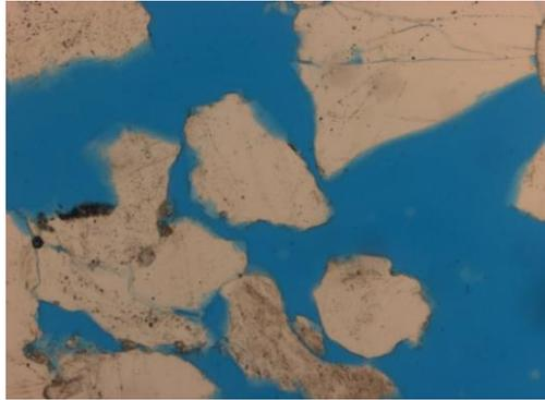
**Figure 9.8** Observed at 10x magnification. In PL, blue dye represents the open pore spaces in the thin section, estimating about 10% porous overall
