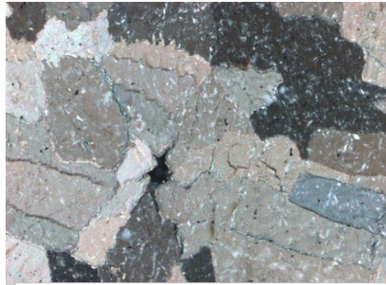
**Figure 10.2** Observed at 10x magnification. In XN, elongated and anhedral calcite grains. Grown together acting as cementing material.
