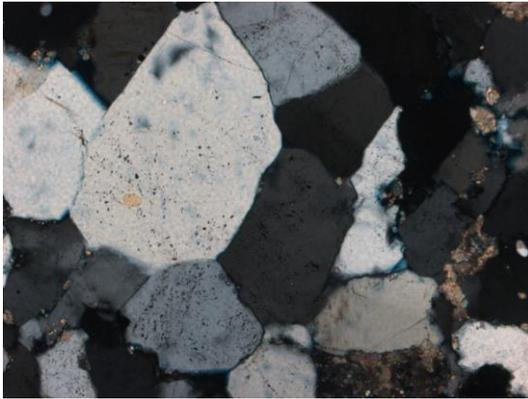
**Figure 4.1** Observed at 10x magnification. In XPL, subhedral, undulose quartz gains. Exhibits quartz growth that results in slight deformation.
