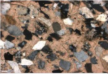
This image shows quartz grains cemented by calcite. (10x, XN)
