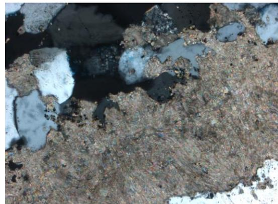
**Figure 10.6** Observed at 10x magnification. In XN, globular calcite overgrown and interspersed with subhedral quartz.
