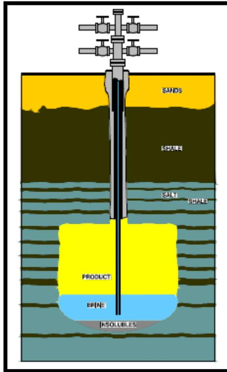
Figure 7. Schematic diagram of a salt cavern (Nelson and others, 2011).
