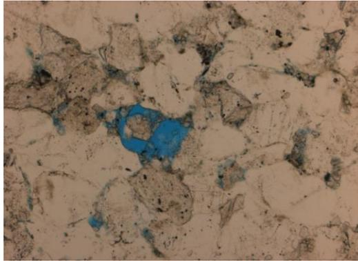
**Figure 8.8** Observed at 10x magnification. In PL, blue dye represents the open pore spaces in the thin section, estimating 5% porosity overall.
