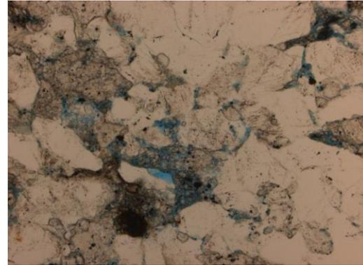
**Figure 8.10** Observed at 10x magnification. In PL, blue dye represents the open pore spaces in the thin section, estimating 5% porosity overall.
