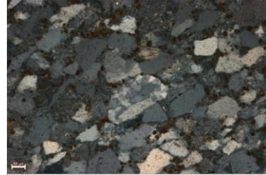
This image shows polycrystalline quartz as well as subhedral, monocrystalline quartz grains.
