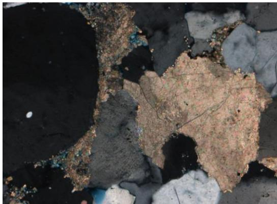
**Figure 6.4** Observed at 10x magnification. In XN, globular calcite grain and calcite cementing material in between subhedral quartz grains.
