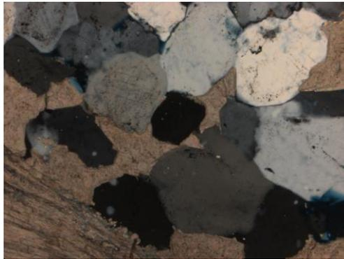
**Figure 9.4** Observed at 10x magnification. In XN, grown calcite cementing together subhedral undulose quartz.
