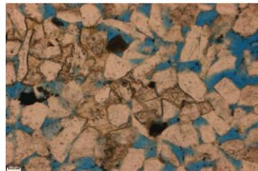
The subhedral grains in this image is shown with blue epoxy filling the pore space. (10x, PPL)
