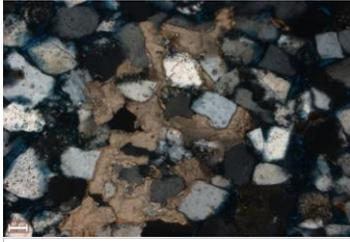
The subangular and subrounded quartz grains in this image are cemented by calcite grains. (10x, XN)
