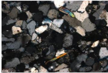
Two grains of birefringent muscovite are embedded in a matrix of intergrown quartz.
