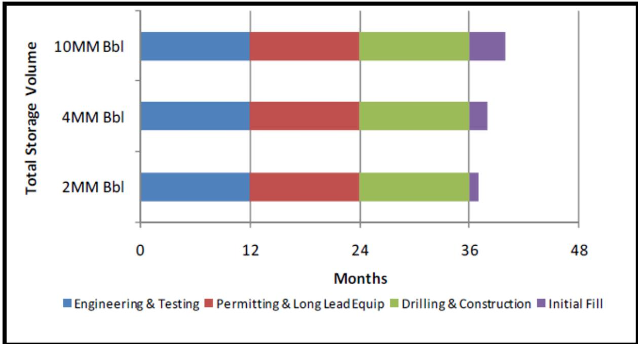
Figure 9. ROM timeline for construction of reservoir storage (Nelson and others, 2011).
