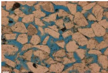
The blue epoxy in this image shows the pore space in the sample. (10x, PPL)
