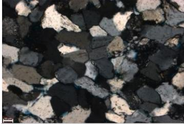
The subhedral quartz grains in this image are intergrown. Some sedimentary rock fragments are also shown.
