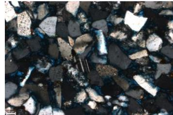
The albite twinning in this image shows the presence of plagioclase feldspar. The feldspar is surrounded by subhedral quartz grains and pore space.
