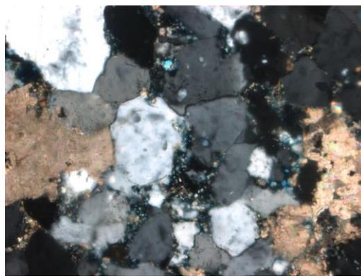
**Figure 11.4** Observed at 10x magnification. In XN, subhedral quartz grains grown with anhedral and slightly deformed calcite grains and calcareous cementing material.
