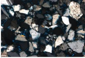
This image shows quartz grains of different sizes. Some sedimentary rock fragments are shown as well. (10x, XN)
