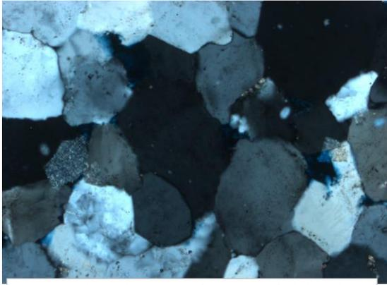
**Figure 10.1** Observed at 10x magnification. In XN (unbalanced light), subhedral undulose quartz grains grown and cemented together.
