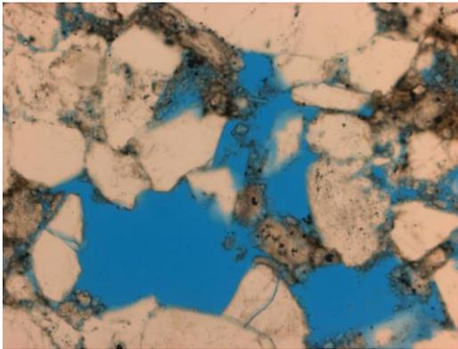
**Figure 11.9** Observed at 10x magnification. In PL, the blue dye represents the open pore spaces in the thin section, estimating about 11% porous overall.
