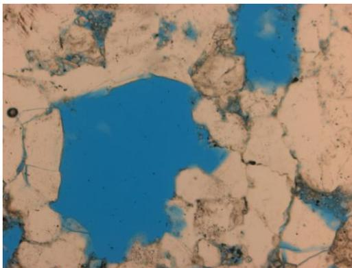
**Figure 11.11** Observed at 10x magnification. In PL, the blue dye represents the open pore spaces in the thin section, estimating about 11% porous overall.
