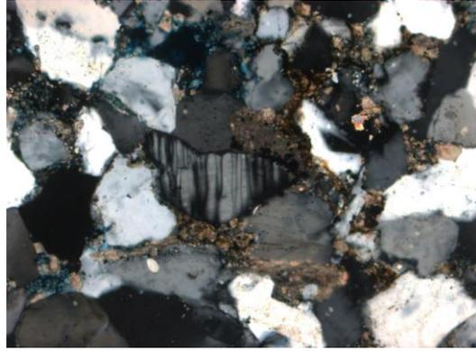
**Figure 11.2** Observed at 10x magnification. In XN, anhedral quartz grain with intergrown calcite cementing material. Also present is a anhedral grain of plagioclase exhibiting albite twinning.
