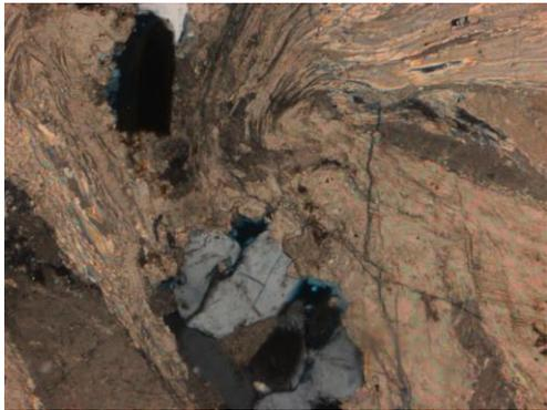
**Figure 9.3** Observed at 10x magnification. In XN, large cumulate of deformed calcite, overgrown on quartz grains.
