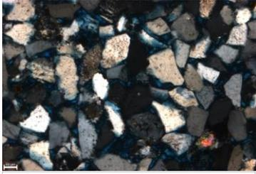
This image shows subangular quartz grains and pore space. (10x, XN)
