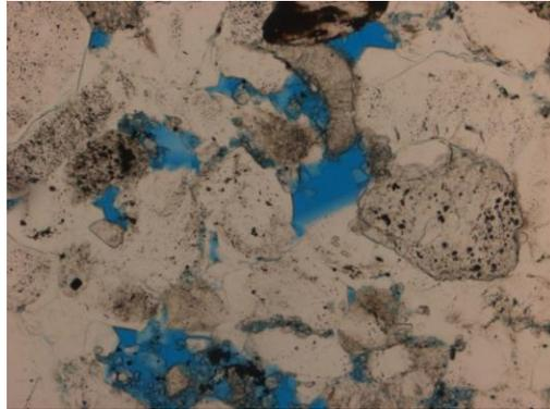
**Figure 7.8** Observed at 10x magnification. In PL, the blue dye represents the open spaces in the thin section, estimating to about 8% porosity overall.
