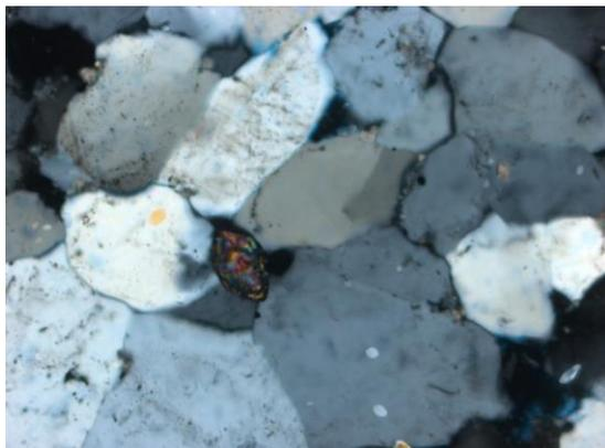
**Figure 10.5** Observed at 10x magnification. In XN, subhedral and slightly intergrown quartz grains with a small grain of deformed
