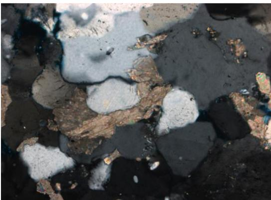
**Figure 6.5** Observed at 10x magnification. In XN, Deformed quartz grains with some globular calcite grains.
