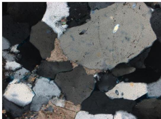
**Figure 6.6** Observed at 10x magnification. In XN, quartz grains being cemented by both quartz growth and carbonate material calcite.
