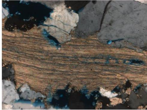
**Figure 9.2** Observed at 10x magnification. In XN, deformed elongated grain of calcite grown in between subhedral quartz grains.
