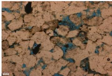
Blue epoxy in this image shows the pore space in this sample.
