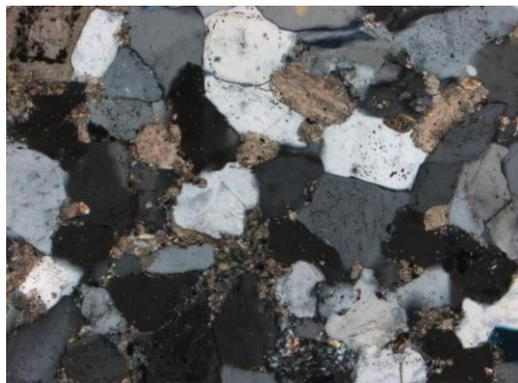
**Figure 8.6** Observed at 10x magnification. In XN, subhedral undulose quartz with intergrown deformed calcite grains acting as cementing material.
