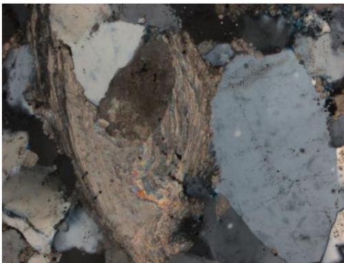
**Figure 7.5** Observed at 10x magnification. In XN, globular, deformed calcite grain surrounded by subhedral grains of quartz.
