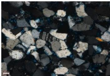
Plagioclase feldspar with albite twinning is shown in this image. Subrounded and subangular quartz grains surround the feldspar.
