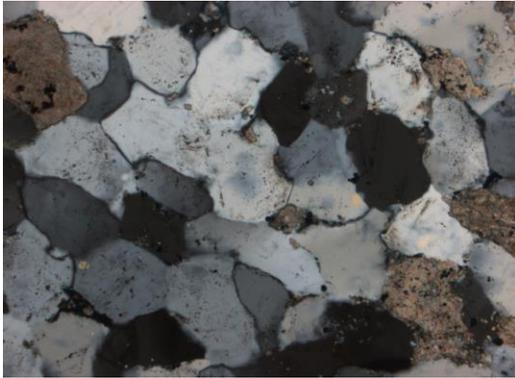
**Figure 8.1** Observed at 10x magnification. In XPN subhedral and slightly deformed, undulose quartz. Slightly intergrown.
