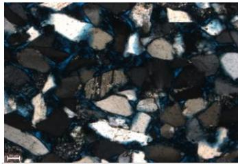
This image shows plagioclase feldspar with albite twinning. Subhedral quartz grains and sedimentary rock fragments surround the feldspar. (10x, XN)
