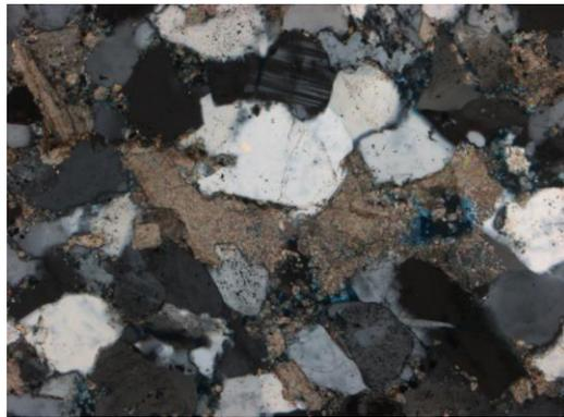
**Figure 8.4** Observed at 10x magnification. In XN, deformed calcite grain grown between deformed and subhedral quartz grains.
