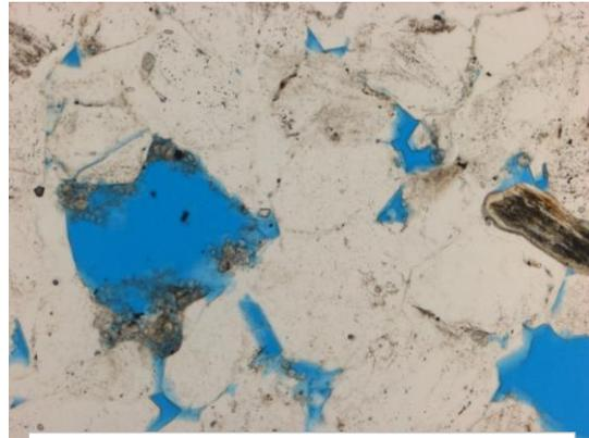
**Figure 10.8** Observed at 10x magnification. In PL, the blue dye represents the open pore spaces in the thin section, estimating to about 10% porous overall.
