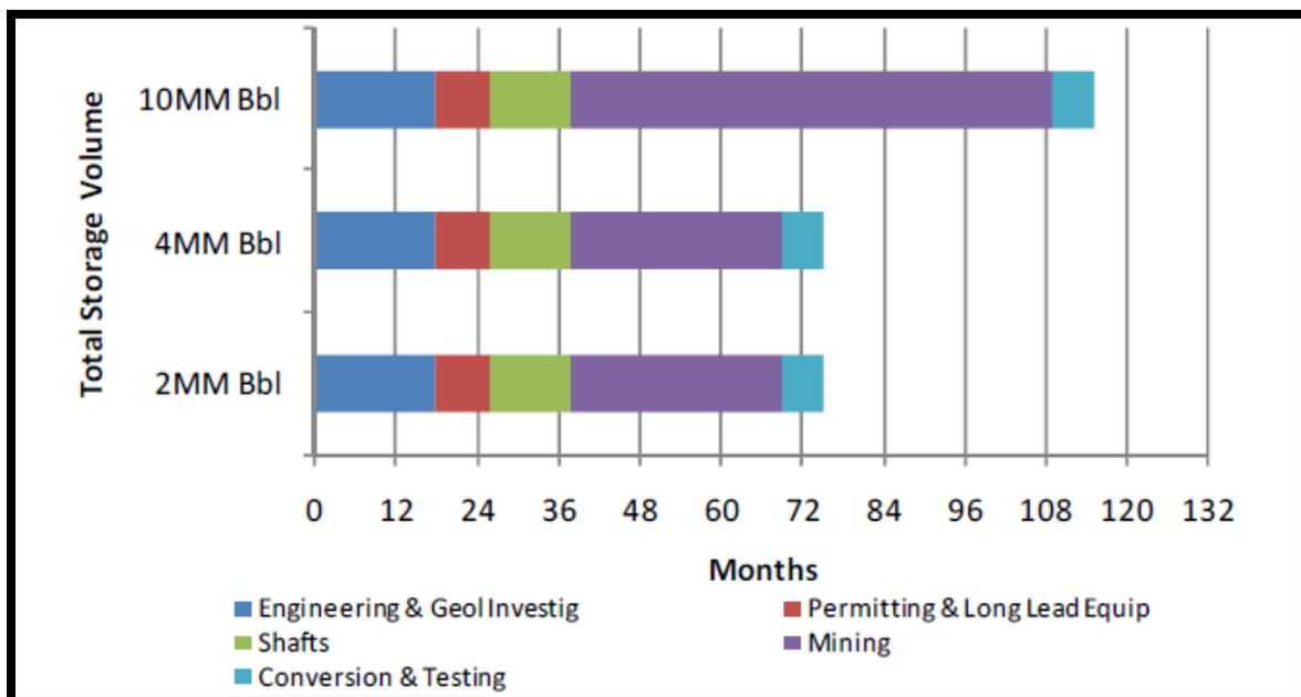
Figure 1. Rough Order of Magnitude (ROM) timeline for construction of a mined-rock cavern.
