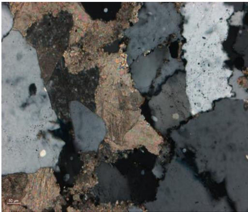
**Figure 3.3** Observed at 10x magnification. In XN, Anhedral, undulose quartz grains grown with and cemented by anhedral, deformed calcite grains. Also quartz grains exhibit quartz intergrowth. Slight
