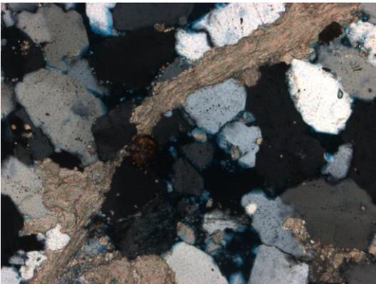
**Figure 4.3** Observed at 10x magnification. In XPL, Anhedral and subhedral undulose quartz . some deform grains from interspersed. Elongated and deformed calcite grains.
