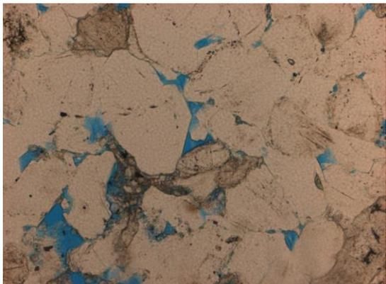
**Figure 6.10** Observed at 10x magnification. In PL, the blue dye indicates the open pores spaces in the thin section. This thin section has an estimated 9% porosity overall.
