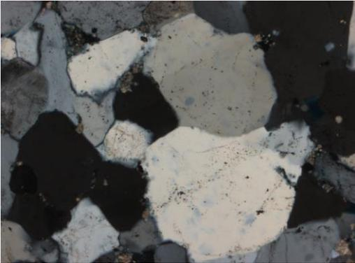
**Figure 7.1** Observed at 10x magnification. In XN, subhedral, intergrown undulose quartz grains. Quartz is acting as cementing material. Some deformed grains.
