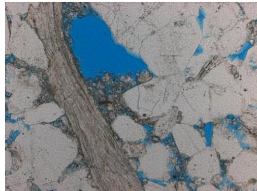
**Figure 5.10** Observed at 10x magnification. In PL, blue dye exhibits the open pore spaces in the thin section. The estimated porosity of the thin section is 11% overall.
