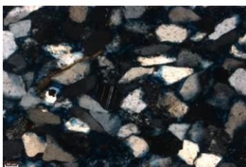
The albite twinning in this image shows plagioclase feldspar surrounded by subhedral quartz grains. (10x, XN)
