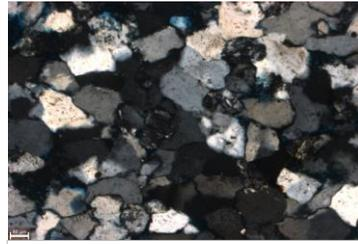
Although slightly difficult to see, this image shows plagioclase feldspar. Intergrown quartz and sedimentary rock fragments are also present in this image.
