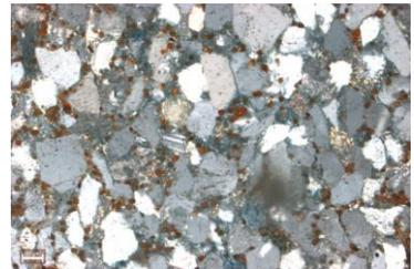
This image shows a small, subangular grain of plagioclase feldspar with albite twinning in a matrix of quartz grains. (10x, XN)
