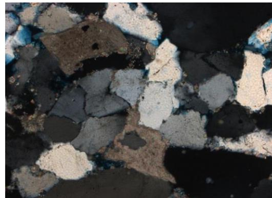
**Figure 5.6** Observed at 10x magnification. In XPL, subhedral and slightly deformed quartz grains with quartz cementing. Also a few deformed calcite grains.
