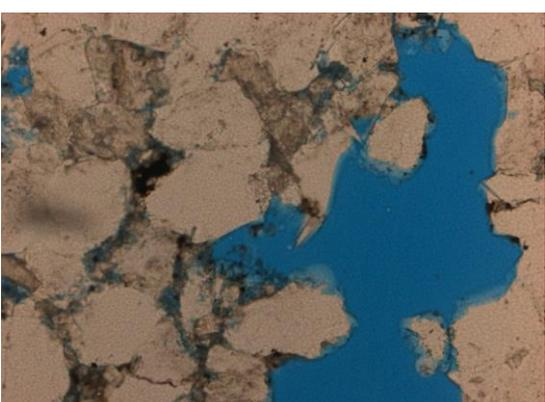
**Figure 6.12** Observed at 10x magnification. In PL, the blue dye indicates the open pores spaces in the thin section. This thin section has an estimated 9% porosity overall.
