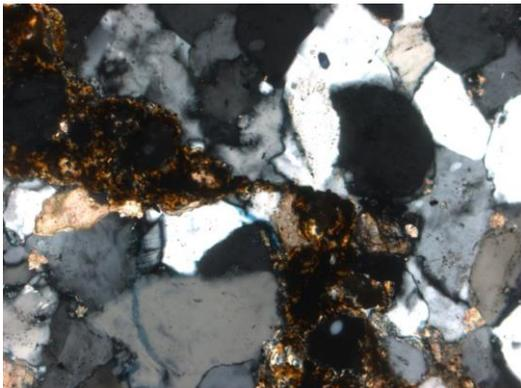
**Figure 11.5** Observed at 10x magnification. In XN, interspersed, subhedral to anhedral undulose quartz grains that are cement calcareous cementing material
