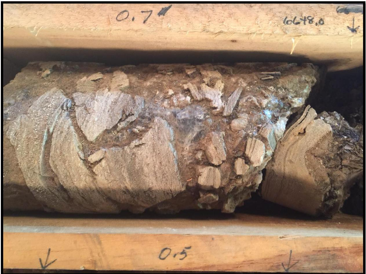
Figure 3. Mix of gray coarse crystalline halite as above and disoriented large (up to 0.8 ft) clasts of thin bedded anhydrite-carbonate plus calcareous shale. Core base is 6,648 ft.
