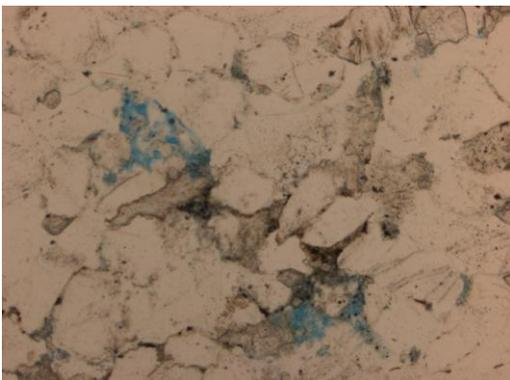
**Figure 8.11** Observed at 10x magnification. In PL, blue dye represents the open pore spaces in the thin section, estimating 5% porosity overall.
