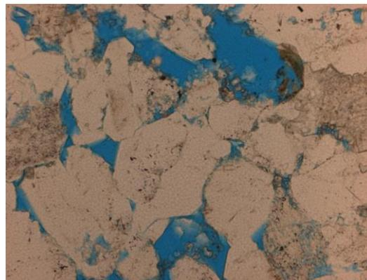
**Figure 4.10** Observed at 10x magnification. In PPL, the blue dye exhibits the open pore spaces in the thin section. Visual estimate of porosity is 13% porous.
