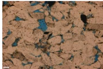
The pore space in these subhedral grains is filled by blue epoxy.
