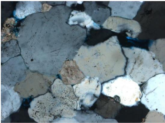
**Figure 10.3** Observed at 10x magnification. In XN, subhedral, undulose quartz grains grown and cemented together.
