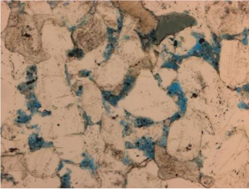
**Figure 11.7** Observed at 10x magnification. In PL, the blue dye represents the open pore spaces in the thin section, estimating about 11% porous overall.
