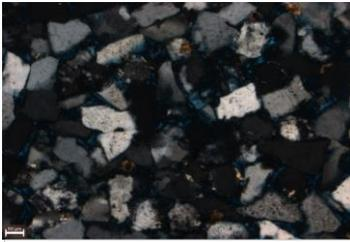
This image shows subangular and subrounded quartz grains with some pore space present as well. (10x, XN)
