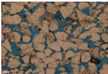
This image shows the pore space in the sample. The blue is the epoxy filling the pore space and the brown is the grains.
