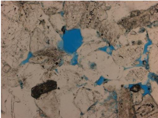
**Figure 7.9** Observed at 10x magnification. In PL, the blue dye represents the open spaces in the thin section, estimating to about 8% porosity overall.
