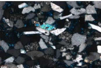
This image shows plagioclase feldspar, a grain of muscovite, sedimentary rock fragments, and subhedral quartz grains. (10x, XN)
