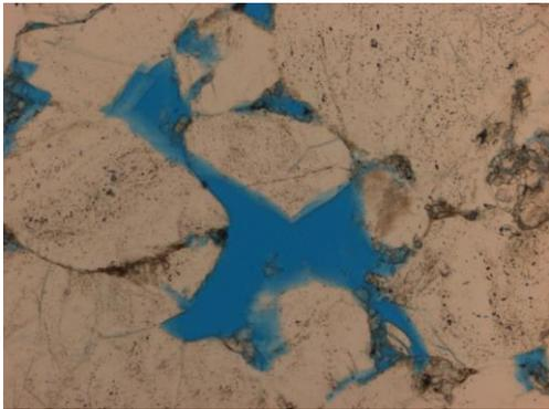
**Figure 9.9** Observed at 10x magnification. In PL, blue dye represents the open pore spaces in the thin section, estimating about 10% porous overall
