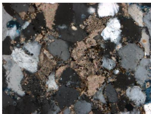
**Figure 7.6** Observed at 10x magnification. In XN, interspersed calcite in between quartz grains. Subhedral quartz grains with calcite cement.
