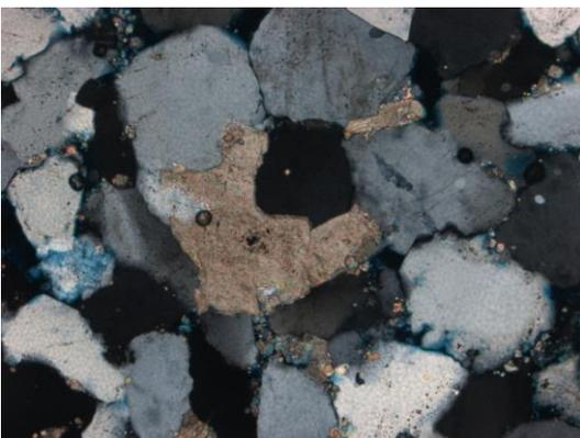
**Figure 4.5** Observed at 10x magnification. In XPL, subhedral undulose quartz grains with some deformation growth with a few deformed calcite grains. Exhibits both quartz and carbonate
