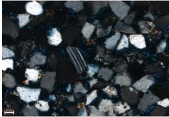
This image shows plagioclase feldspar with albite twinning. Some quartz grains and pore space is shown as well. (10x, XN)
