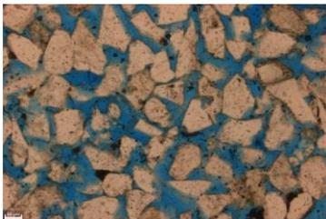
The blue epoxy in this image shows the pore space of the sample. (10x, PPL)
