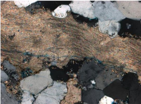
**Figure 6.3** Observed at 10x magnification. In XN, globular grain of calcite with subhedral, subrounded undulose quartz grains.
