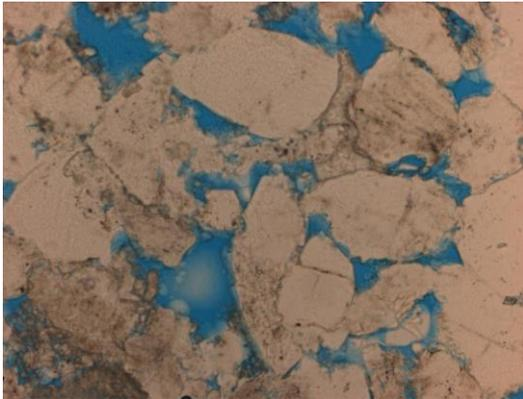
**Figure 4.9** Observed at 10x magnification. In PPL, the blue dye exhibits the open pore spaces in the thin section. Visual estimate
