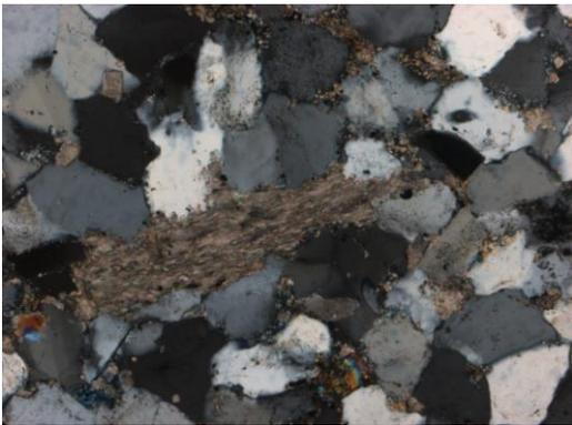
**Figure 8.3** Observed at 10x magnification. In XN, deformed elongated calcite surrounded by subhedral quartz.
