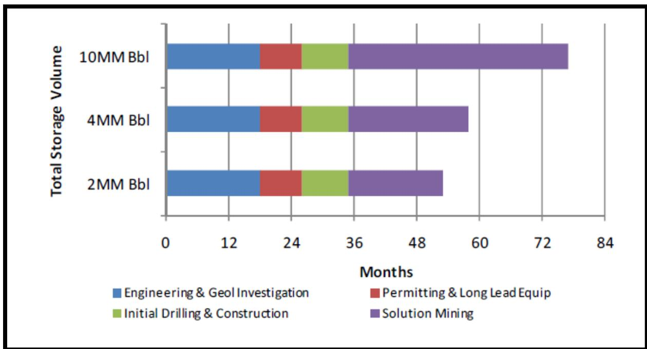
Figure 5. ROM timeline for construction of a salt-brine cavern complex.
