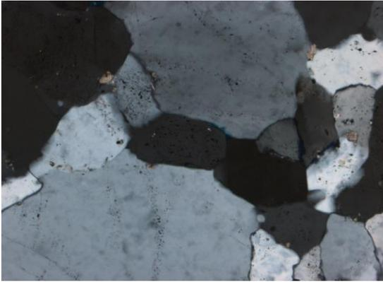
**Figure 6.1** Observed at 10x magnification. In XPN subhedral, intergrown, undulose quartz grains. Quartz is the acting cementing material.
