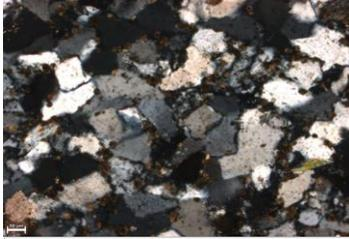
Intergrown quartz grains in this image are covered with iron. (10x, XN)
