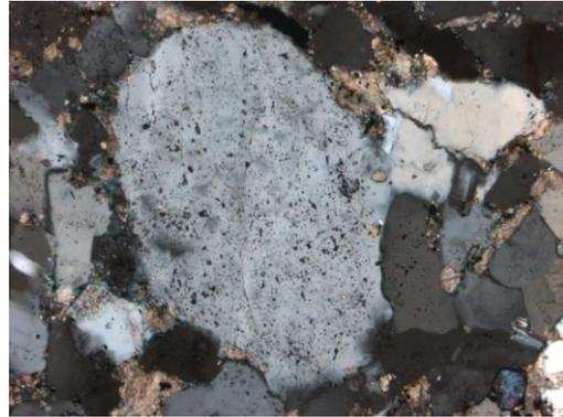
**Figure 8.2** Observed at 10x magnification. In XN, large subhedral quartz grain surrounded by anhedral to subhedral quartz and small amounts of deformed calcite.
