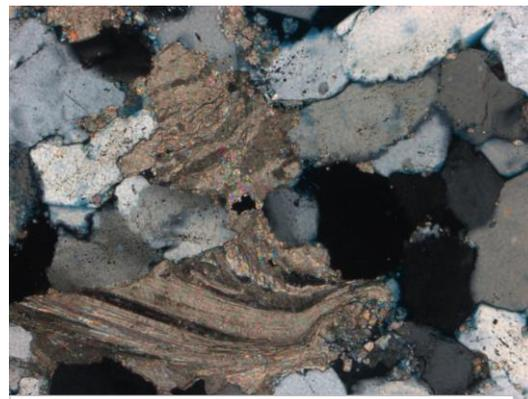
**Figure 4.6** Observed at 10x magnification. In XPL, deformed, globular calcite grain cementing together subhedral, undulose quartz grains..
