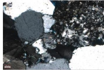
This image shows plagioclase feldspar with albite twinning. Some larger quartz grains and sedimentary rock fragments are present as well.
