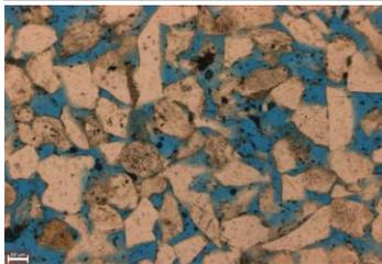
The blue epoxy shows the pore space in this sample. (10x, PPL)
