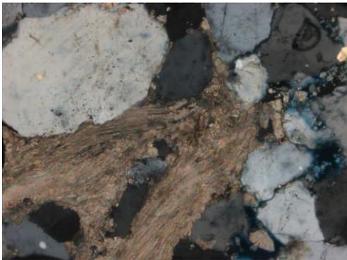
**Figure 9.5** Observed at 10x magnification. In XN, interspersed calcite cementing together subhedral undulose quartz.
