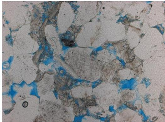
**Figure 5.9** Observed at 10x magnification. In PL, blue dye exhibits the open pore spaces in the thin section. The estimated porosity of the thin section is 11% overall.
