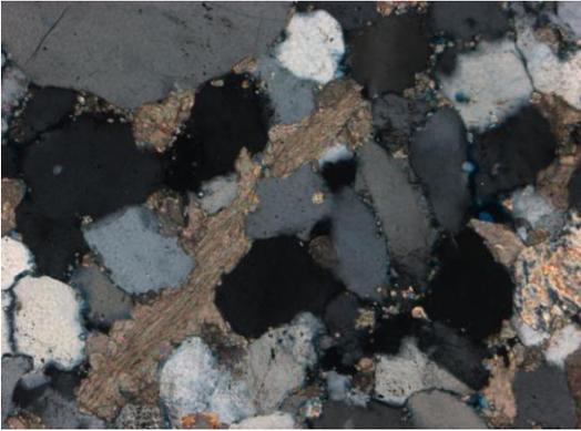
**Figure 5.1** Observed at 10x magnification. In XN, Slightly deformed undulose quartz grains with semi-elongated calcite grain
