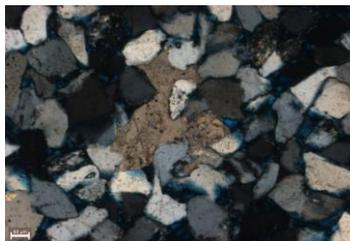
This image shows a grain of anhydrous calcite surrounded by smaller, subhedral quartz grains.
