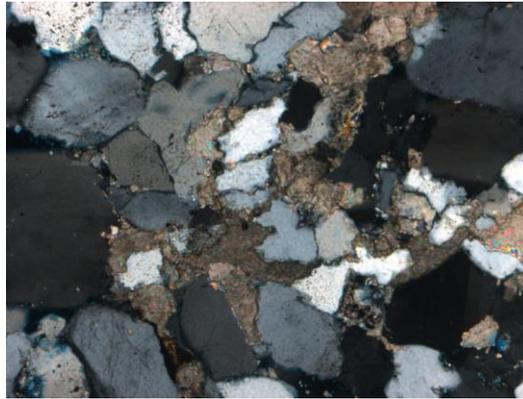
**Figure 4.8** Observed at 10x magnification. In XPL, Deformed, undulose quartz grains with calcareous cementing materials.
