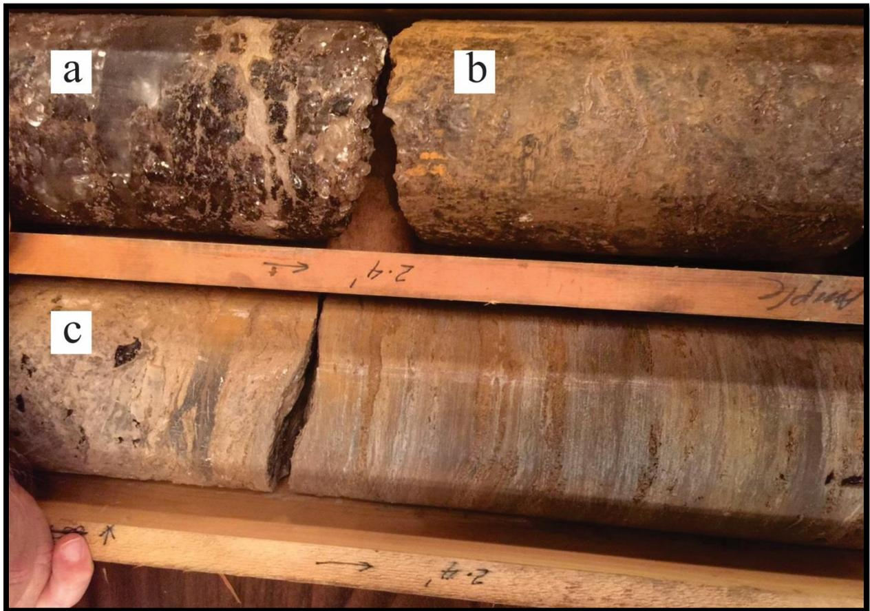
**Figure 1. a: Coarse halite crystals with evenly disseminated black anhydrite pieces that give the section a dark gray color; b: post-lithification fracture includes some salt crystals along the fracture zone; c: brown-gray calcareous shale, thinly laminated, sometimes wavy, partially replaced by salt and pepper carbonate(?)-anhydrite mixture. The shale is interbedded with the carbonate-anhydrite beds.**
