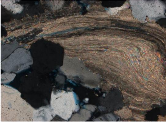
**Figure 6.7** Observed at 10x magnification. In XN, massive globular calcite grain with some slightly deformed undulose quartz grains.
