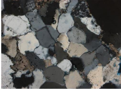
**Figure 7.2** Observed at 10x magnification. In XN, subhedral, undulose quartz grains. Overgrown quartz grains. Also present, subhedral to euhedral calcite grains.
