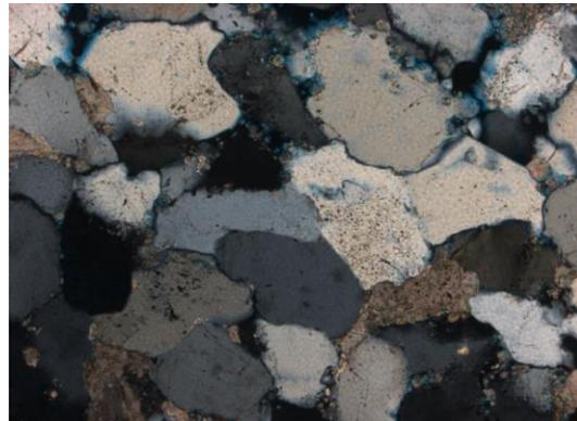
**Figure 5.4** Observed at 10x magnification. In XN, subhedral and slightly deformed undulose quartz. Some interspersed grains.
