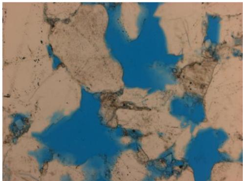
**Figure 9.11** Observed at 10x magnification. In PL, blue dye represents the open pore spaces in the thin section, estimating about 10% porous overall
