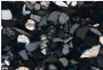
This image shows a grain of subhedral muscovite along with quartz grains, pore space, and sedimentary rock fragments. (10x, XN)
