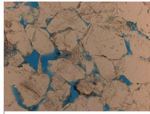
**Figure 4.12** Observed at 10x magnification. In PPL, the blue dye exhibits the open pore spaces in the thin section. Visual estimate of porosity is 13% porous.
