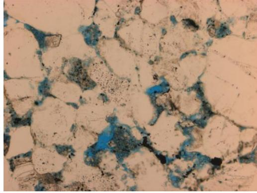
**Figure 11.8** Observed at 10x magnification. In PL, the blue dye represents the open pore spaces in the thin section, estimating about 11% porous overall.
