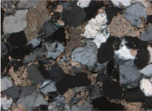
**Figure 8.7** Observed at 10x magnification. In XN, deformed calcite grains in between quartz, acting as cementing material. quartz appears to be anhedral to subhedral.
