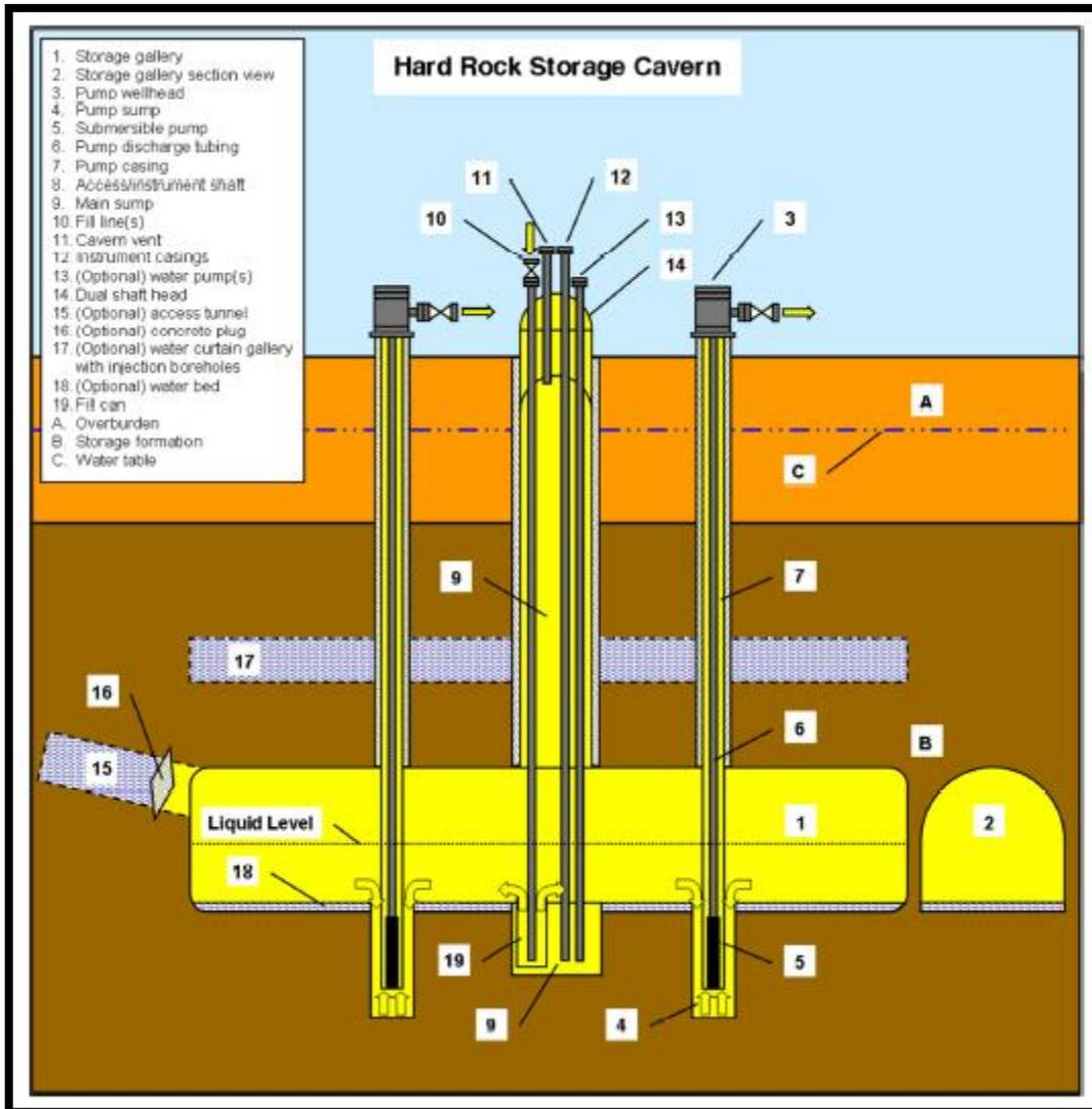
**Figure 3. Schematic (cross section view) design of a mined-rock cavern.**
