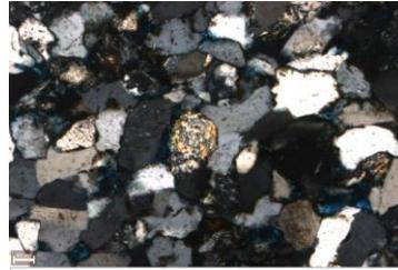
This image shows a sedimentary rock fragment with iron present in the grain. Intergrown quartz grains surround the sedimentary rock fragment.
