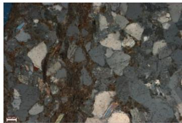
The subhedral quartz grains in this image are cemented by calcite. Some grains of birefringent muscovite are also present. (10x, XN)
