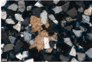
The calcite in this image cements quartz grains. (10x, XN)
