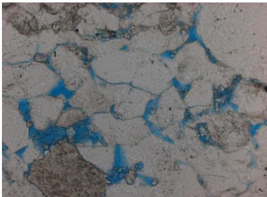
**Figure 5.11** Observed at 10x magnification. In PL, blue dye exhibits the open pore spaces in the thin section. The estimated porosity of the thin section is 11% overall
