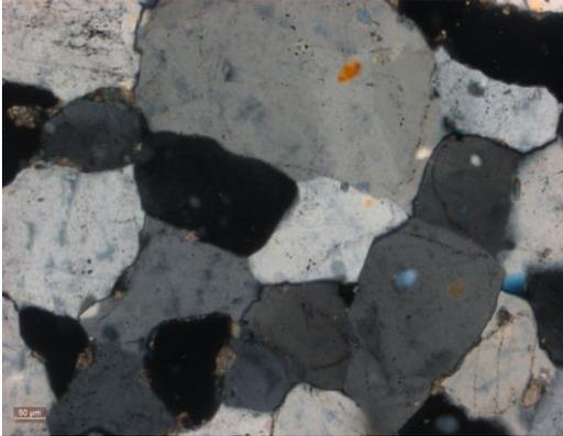
**Figure 3.1** Observed at 10x magnification. In XN, subhedral undulose quartz grains cemented together by quartz growth
