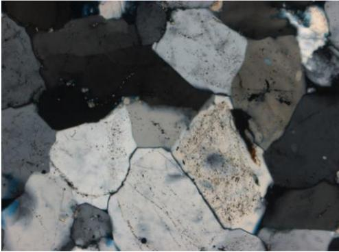
**Figure 9.1** Observed at 10x magnification. In XN, subhedral undulose quartz that is also acting as cementing material from growth.
