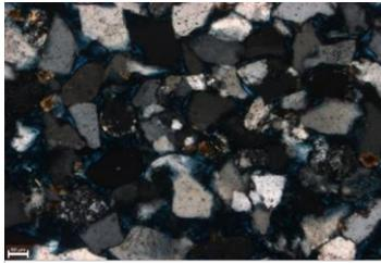
Subhedral quartz grains are shown in this image along with some polycrystalline quartz grains and sedimentary rock fragments. (10x, XN)
