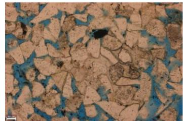
This image shows the porosity of the sample. The light-brown, subangular grains are surrounded by blue epoxy. (10x, PPL)
