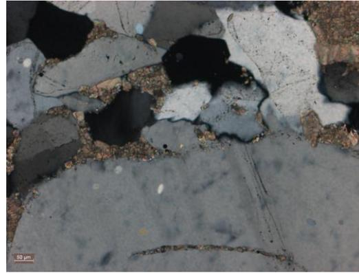
**Figure 3.2** Observed at 10x magnification. In XN, anhedral, undulose quartz grains that is calcareously cemented. Also quartz grains show example of overgrowth.
