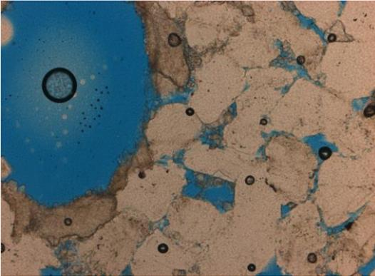
**Figure 5.7** Observed at 10x magnification. In PL, blue dye exhibits the open pore spaces in the thin section. the estimated porosity of the thin section is 11% overall
