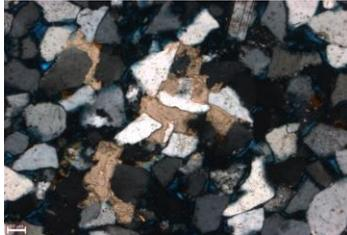
This image shows subhedral calcite along with quartz grains and some pore space. (10x, XN)
