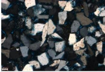
Subangular and subrounded quartz grains are shown in this image. (10x, XN)
