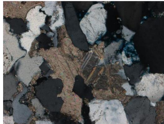
**Figure 4.4** Observed at 10x magnification. Deformed undulose quartz grains with deformed calcite grains acting as cementing material. Calcite exhibits some lamellar twinning.
