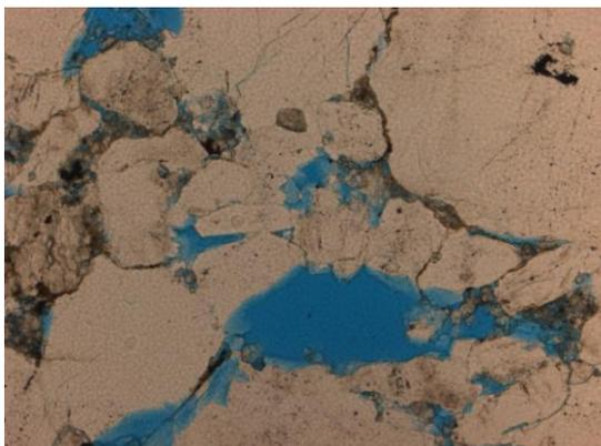
**Figure 6.11** Observed at 10x magnification. In PL, the blue dye indicates the open pores spaces in the thin section. This thin section has an estimated 9% porosity overall.
