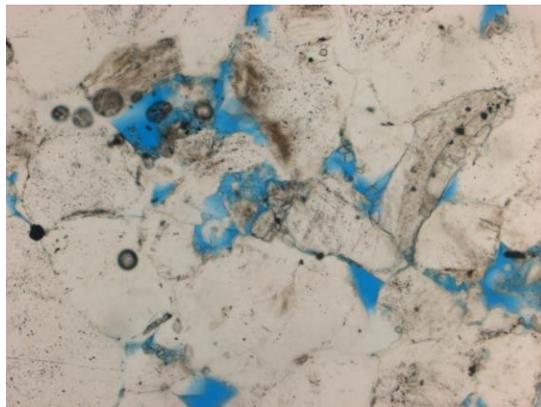
**Figure 10.10** Observed at 10x magnification. In PL, the blue dye represents the open pore spaces in the thin section, estimating to about 10% porous overall.
