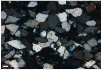
This image shows subrounded and subangular quartz grains with some intergrowth and some pore space visible. Colored muscovite can be seen in the top right corner as well.
