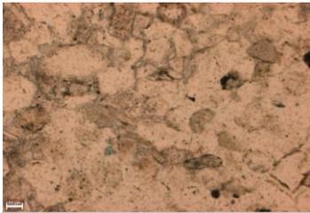
There is hardly any blue epoxy in this image but the blue epoxy that is visible shows the pore space in the sample. (10x, PPL)
