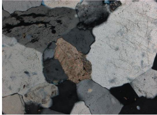
**Figure 6.2** Observed at 10x magnification. In XPL, subhedral undulose quartz grains and a subhedral calcite grain.
