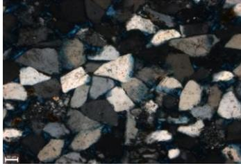
This image shows subangular and subrounded quartz grains with some pore space visible. (10x, XN)
