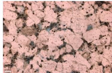
The pore space in this image is filled with blue epoxy. (10x, PPL)
