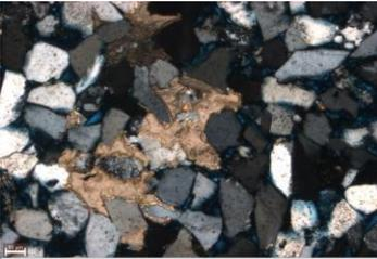
This image shows calcite cementing smaller quartz grains and sedimentary rock fragments. (10x, XN)
