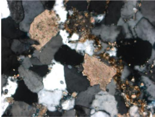
**Figure 11.3** Observed at 10x magnification. In XN, anhedral to subhedral, quartz grains with subhedral calcite grains and intergrown calcareous cementing material
