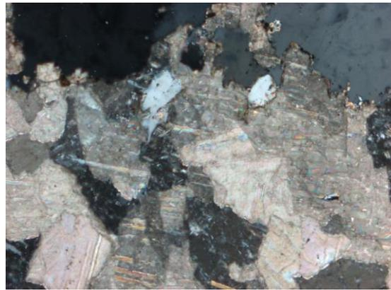
**Figure 10.4** Observed at 10x magnification. In XN, globular calcite with lamellar twinning with a few overgrown quartz grains.
