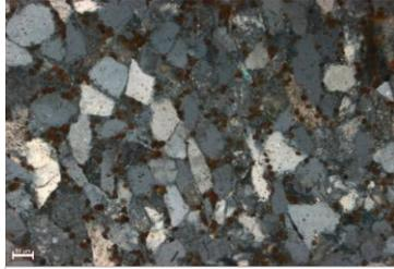
The subangular and subrounded quartz grains in this image. Some iron is shown here as well. (10x, XN)
