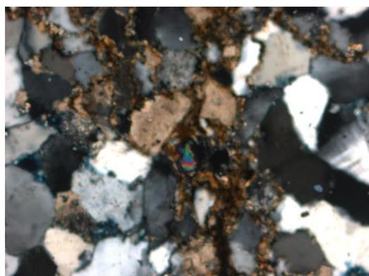
**Figure 11.6** Observed at 10x magnification. In XN, subhedral undulose quartz grains overgrown and cemented with calcareous material and calcite in between.
