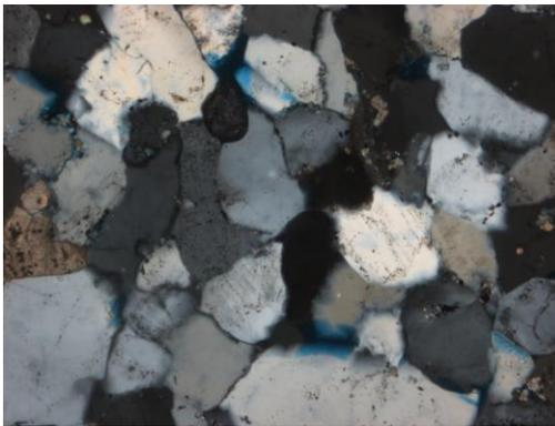
**Figure 7.3** Observed at 10x magnification. In XN, anhedral to subhedral, undulose quartz grains. Quartz is the cementing
