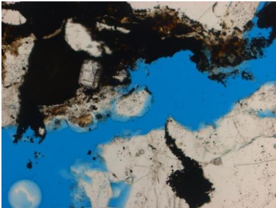
**Figure 10.9** Observed at 10x magnification. In PL, the blue dye represents the open pore spaces in the thin section, estimating to about 10% porous overall.
