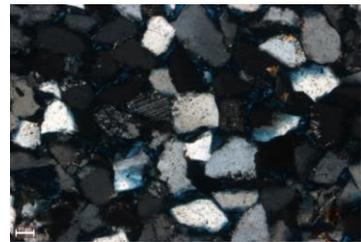
Plagioclase feldspar with albite twinning is surrounded by subhedral quartz grains in this image. (10x, XN)
