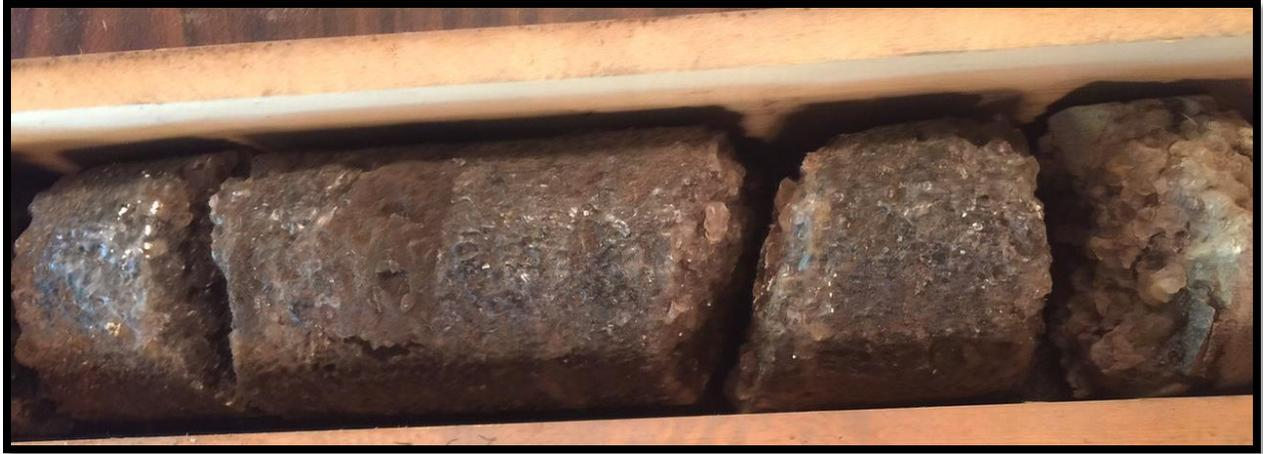
Figure 2. Uniformly coarse (0.25-0.5 inch) halite crystals with evenly disseminated black anhydrite pieces, which give the section a dark gray color.
