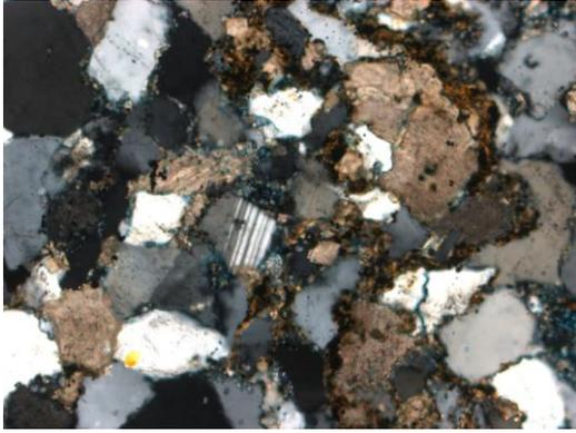
**Figure 11.1** Observed at 10x magnification. In XN, intergrown , anhedral and deformed quartz and calcite grains. Also present is a small piece of plagioclase.
