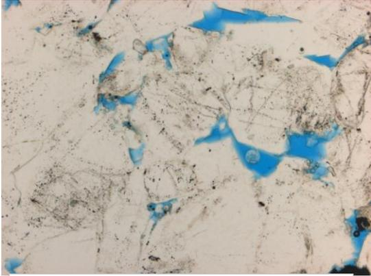
**Figure 10.7** Observed at 10x magnification. In PL, the blue dye represents the open pore spaces in the thin section, estimating
