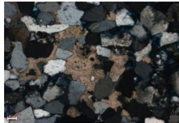
The quartz in this image is cemented by grains of anhydrous calcite.
