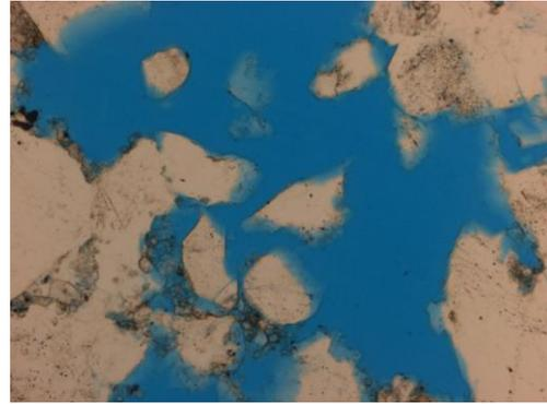
**Figure 9.10** Observed at 10x magnification. In PL, blue dye represents the open pore spaces in the thin section, estimating about 10% porous overall
