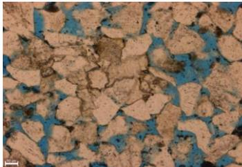
The blue in this image is epoxy used to show pore space in a sample. (10x, PPL)
