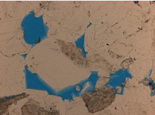
**Figure 6.9** Observed at 10x magnification. In PL, the blue dye indicates the open pores spaces in the thin section. This thin section has an estimated 9% porosity overall.
