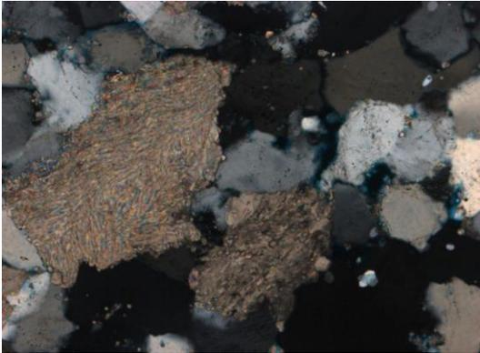
**Figure 5.3** Observed at 10x magnification. In XN, anhedral calcite grain with anhedral to subhedral undulose quartz grains. Quartz intergrowth is evident
