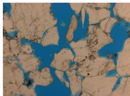
**Figure 9.12** Observed at 10x magnification. In PL, blue dye represents the open pore spaces in the thin section, estimating about 10% porous overall
