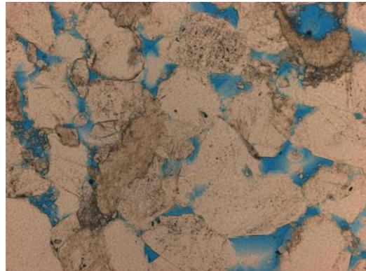
**Figure 5.8** Observed at 10x magnification. In PL, blue dye exhibits the open pore spaces in the thin section. the estimated porosity of the thin section is 11% overall
