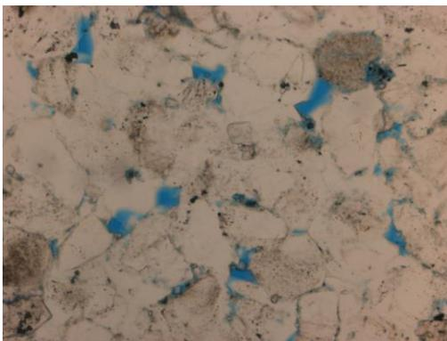
**Figure 7.11** Observed at 10x magnification. In PL, the blue dye represents the open spaces in the thin section, estimating to about 8% porosity overall.
