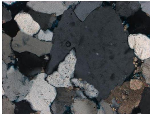
**Figure 4.2** Observed at 10x magnification. In XPL, anhedral to subhedral, undulose quartz. Exhibits quartz intergrowth. Also some deformed calcite grains.
