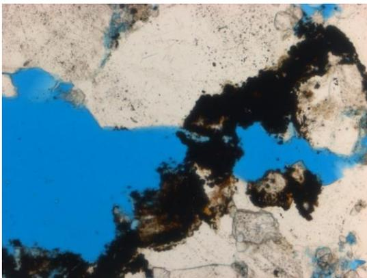
**Figure 10.11** Observed at 10x magnification. In PL, the blue dye represents the open pore spaces in the thin section, estimating to about 10% porous overall.
