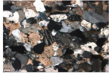
The plagioclase feldspar in this image shows albite twinning surrounded by calcite and intergrown quartz. (10x, XN)
