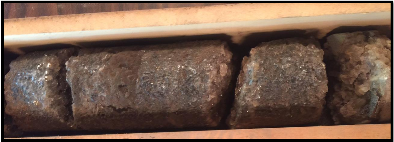
Figure 4-14. Uniformly coarse (0.25-0.5 inch [in]) halite crystals with evenly disseminated black anhydrite pieces, which give the sample a dark gray color.
