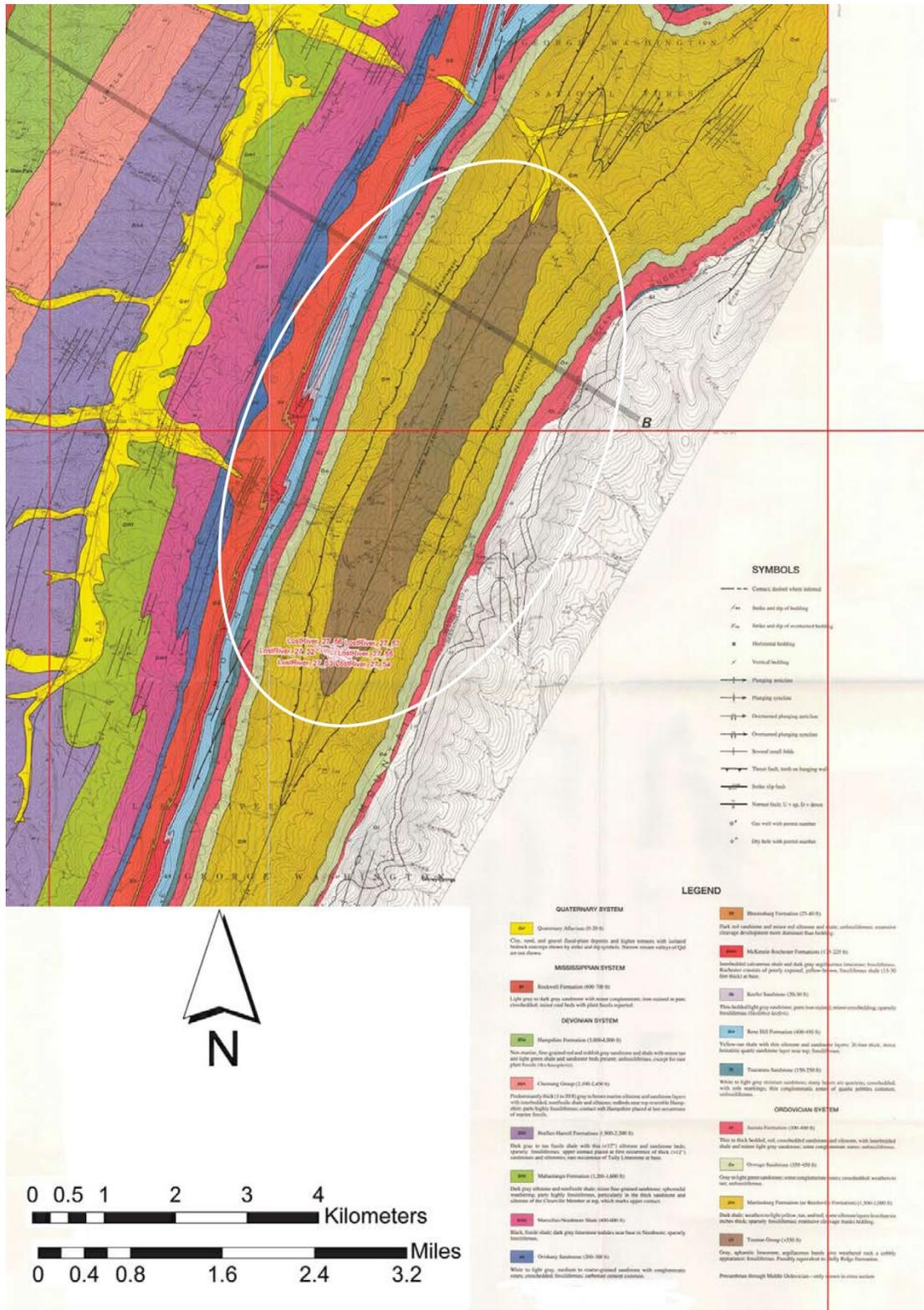
Figure 1-9. Ordovician exposures near Lost River, West Virginia. Exposures are thought to be of the Martinsburg Formation and may be incorrectly mapped as Trenton Group (=Lexington/Trenton Formation of this Study).
