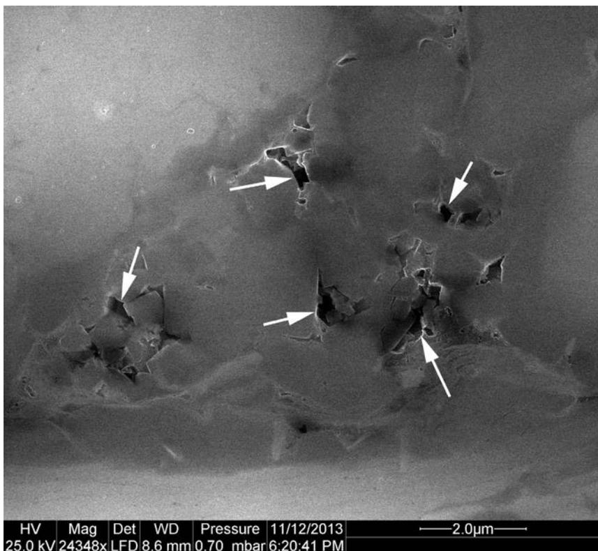
**Figure 7:** White arrows point to open framework pores defined by carbonate grains. Because of abundant early diagenetic carbonate growth and the high carbonate content of the rock, Carbonate Framework Pores appear to be more abundant in this sample when compared to previous samples (170-655 feet).
