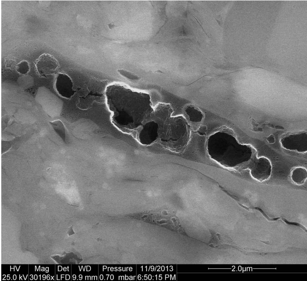
**Figure 7:** An elongate space filled with porous OM/bitumen, very well developed large (multi-micron) bubble pores. These show pore throats at depth and are most likely interconnected throughout the sample. White rims of large pores are again a charging artifact (avoidable, but harmless, allows better image quality elsewhere). OM porosity like this is typical for good reservoir facies in the Eagleford and Haynesville shales.
