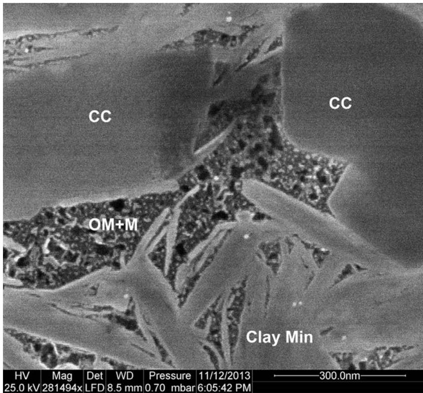
**Figure 6:** Close-up of Fig. 5. Shows that in this instant the OM filled areas are not simply OM plus pores, but OM that is finely mingled with mineral matter (brighter gray spots) and also contains pores (dark gray to black spots). These mineral grains were probably carried with the hydrocarbon liquids (now bitumen) that entered the original pore spaces.
