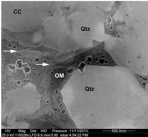
**Figure 7:** Another example of pore spaces defined by diagenetic quartz, and infilled with diagenetic clays and bitumen with OM bubble and foam pores.
