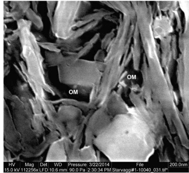
**Figure 3.-.-.** Organic matter within interstitial spaces. Left – Darker area (arrows) marks an area where clays and OM are intermingled (OM “invaded” during hydrocarbon generation). Right – Close-up that shows OM between clay mineral flakes.
