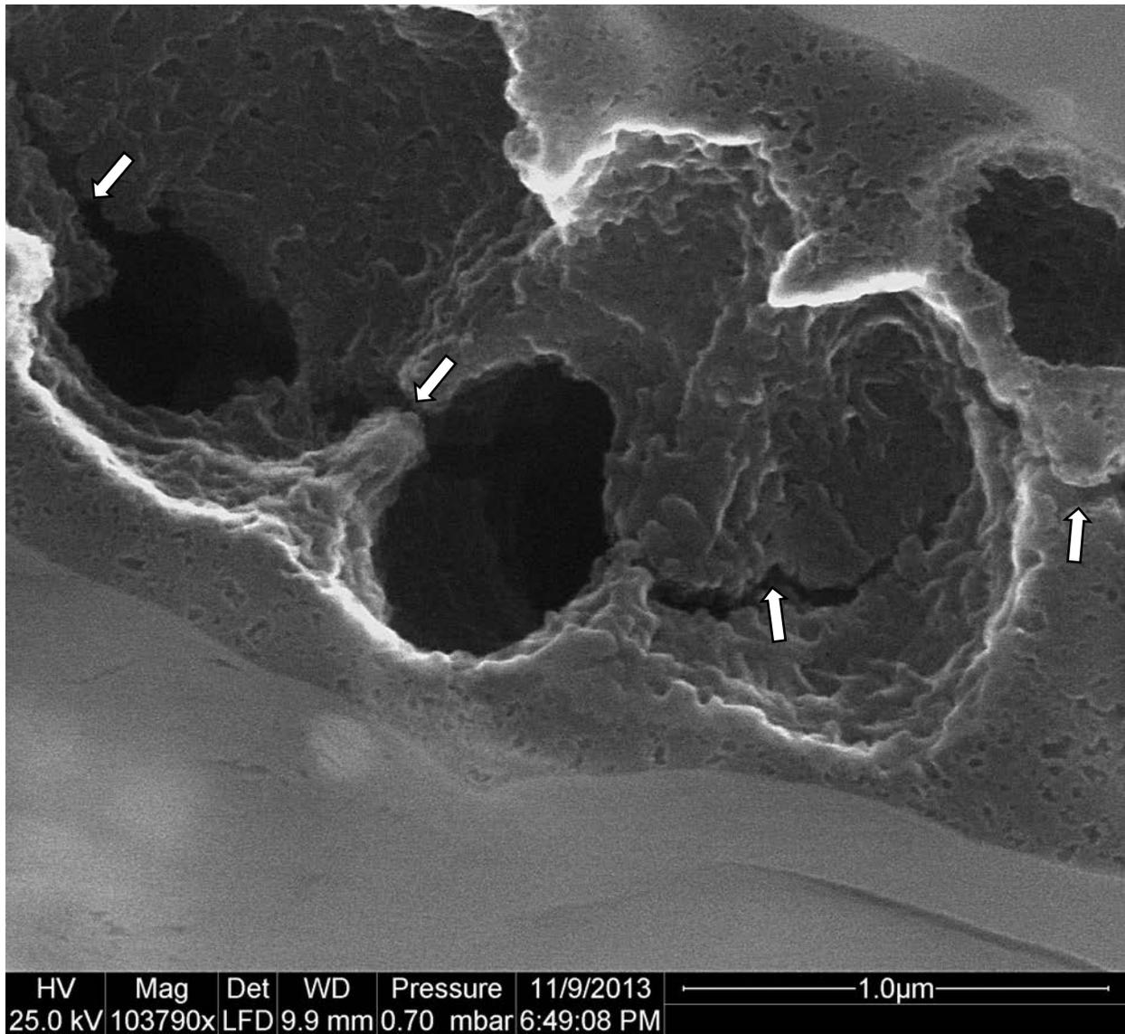
**Figure 8:** Close-up from Fig. 7. Shows the foam pores (gas storage) in the bitumen matrix that contains the larger bubble pores (gas transport). At this magnification we can identify an abundance of foam pores in the 10 nm or larger size range. The white arrows point to a fracture that roughly parallels the OM in this area, most likely a result of sample expansion due to removal of confining pressure.
