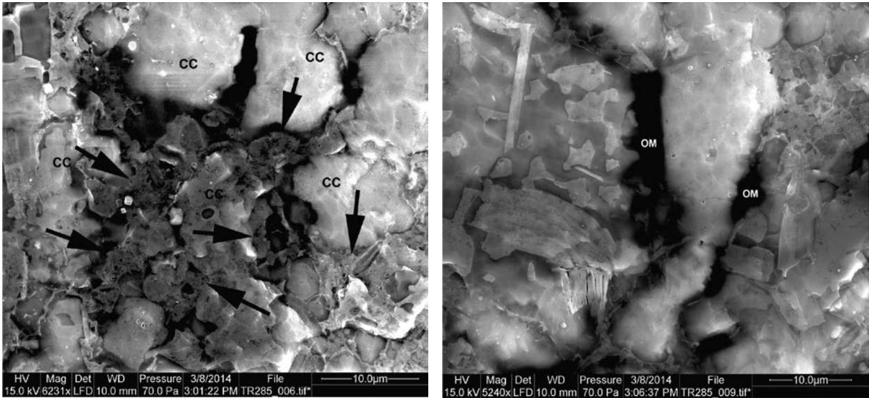
**Figure 4. Left – A fabric overview. Large calcite grains (CC) have squeezed areas between them (arrows) where most of the quartz and clays and OM occur. Right – Closer view of tight interlocking fabric with amorphous OM in interstitial locations. These two OM spots did not show pore development.**
