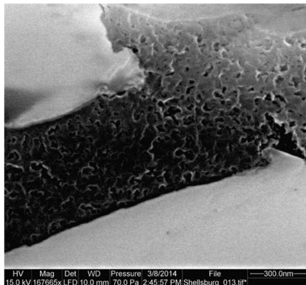
**Figure 3. Left – View of interstitial OM between diagenetic quartz grains. The way the OM “invades” this space suggests that it came in as a fluid/hydrocarbon liquid. It is probably some sort of bitumen now. Right – Close-up of this OM that shows pervasive small pores of the “foam” type, ranging in size from 10-100 nm. This is the way the OM in this sample typically looks like.**
