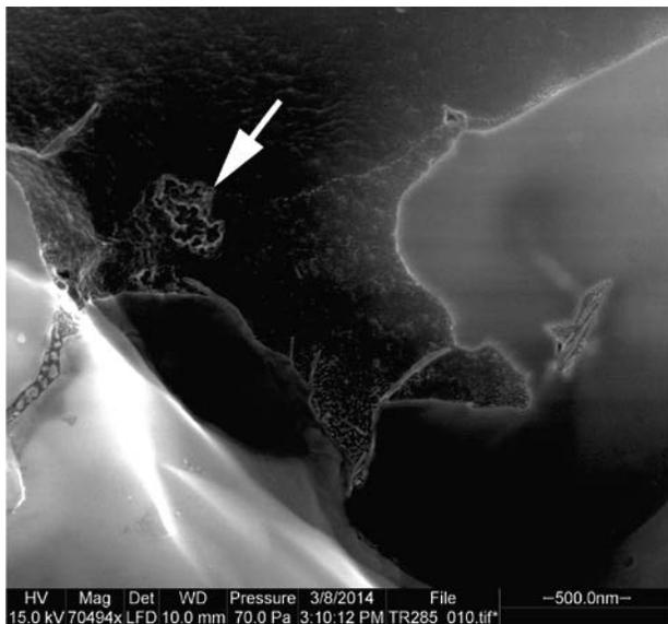
**Figure 5. Close-up of another interstitial OM pocket. This one shows some pore development (arrow), but it is not pervasive. There is development of a “dimpled” texture on the OM, suggesting that it is still soft OM/bitumen, and that we are still within the oil window.**
