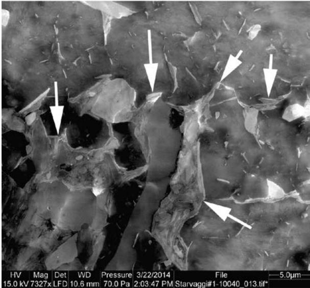
**Figure 14. Typical fabric with large calcite crystals (with mineral inclusions) and interstitial quartz, clays (arrows), and OM pockets.**
