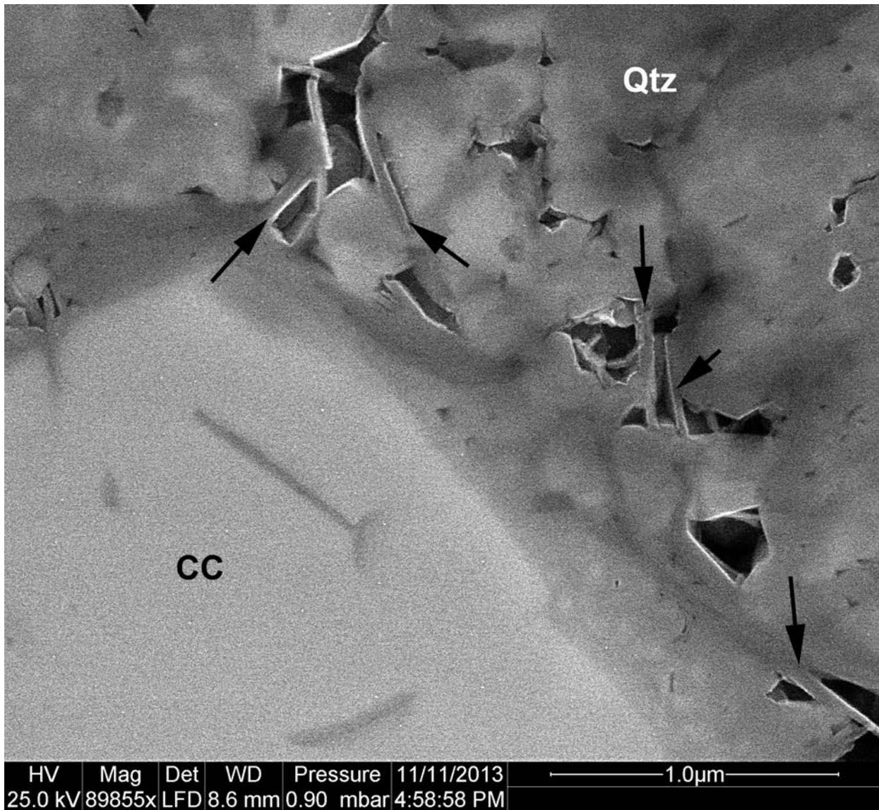
**Figure 4:** Framework pores between diagenetic quartz grains (Qtz), partly also defined by (most likely diagenetic) clay flakes (black arrows). CC=calcite. In this sample these kinds of framework pores are common, but OM porosity still dominates overall porosity.
