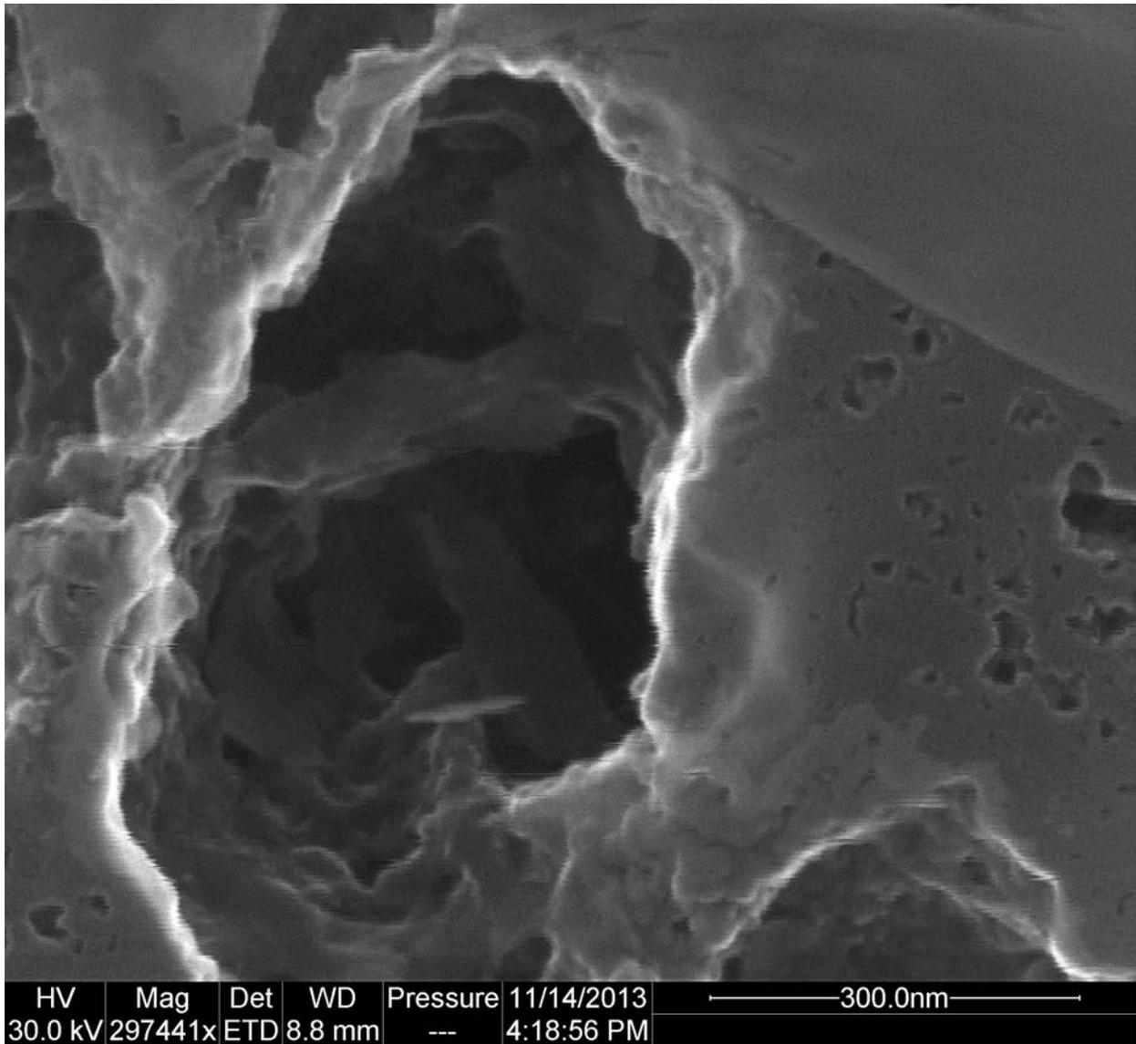
**Figure 6:** Closeup of pores in OM. Shows in depth pore throats that are probably interconnected. These pores most likely are critical to reservoir performance.
