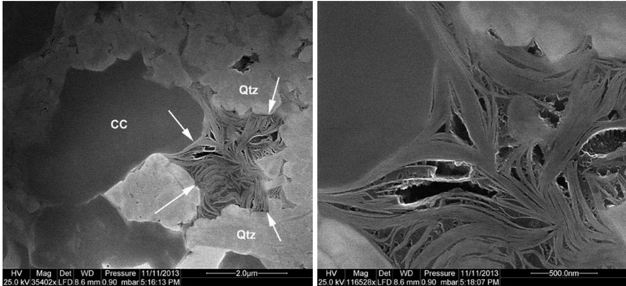
**Figure 6:** Example where a late diagenetic pore defined by calcite (cc) and diagenetic quartz grains (Qtz) is filled by clays (probably diagenetic) that form an open framework whose pores were subsequently filled by organic matter (bitumen). Heating of the bitumen produced the observed OM pores in the bitumen fill.
