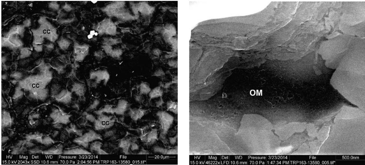
**Figure 12. Left – Typical fabric (overview, backscatter image). The light gray grains are calcite (CC), and in between them are mainly diagenetic quartz (some detrital inclusions), clays, and some OM. Right – Pocket of amorphous OM in an interstitial area that shows development of mainly small “foam” pores (10-50 nm mostly), and a few larger pores that may mark the onset of bubble pore formation.**
