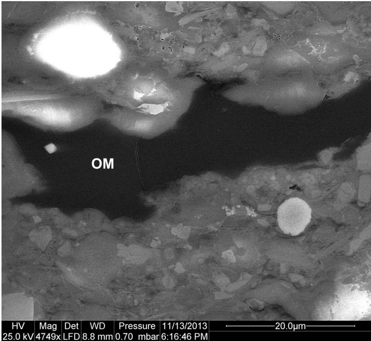
**Figure 7:** A piece of organic matter (probably plant derived ) within the silicate bearing shale matrix. This structured OM (cross linked) does not show pore development, even at high maturity levels. There is not too much of this type of OM visible (in relative terms), and its presence most likely does not have a serious negative effect on overall porosity and permeability.
