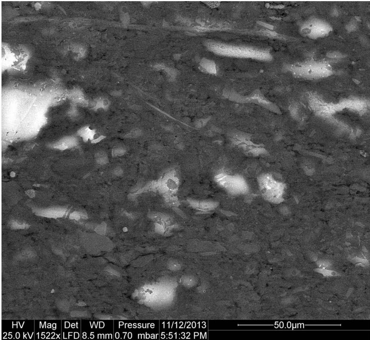
**Figure 2:** Mid-level overview of shale fabric (SEM image). Bright areas are characterized by continuous calcite cement (brightness due to charging). The fabric consists largely of a mingling of calcite grains, quartz grains, and clays and organic matter (dark-black areas) that are crowded together in interstitial areas. A few thin calcareous slivers (light gray) are fossil shell material.
