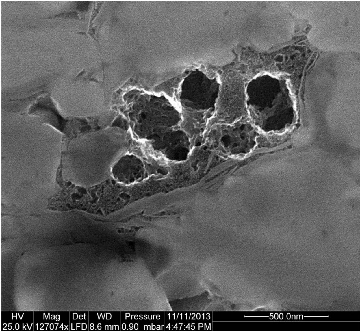
**Figure 3:** Close-up of organic matter pore fill from Fig. 2. Note large bubble pores with at depth pore throats and connectivity, and abundant foam pores in OM matrix. OM most likely bitumen infill of originally open pores.
