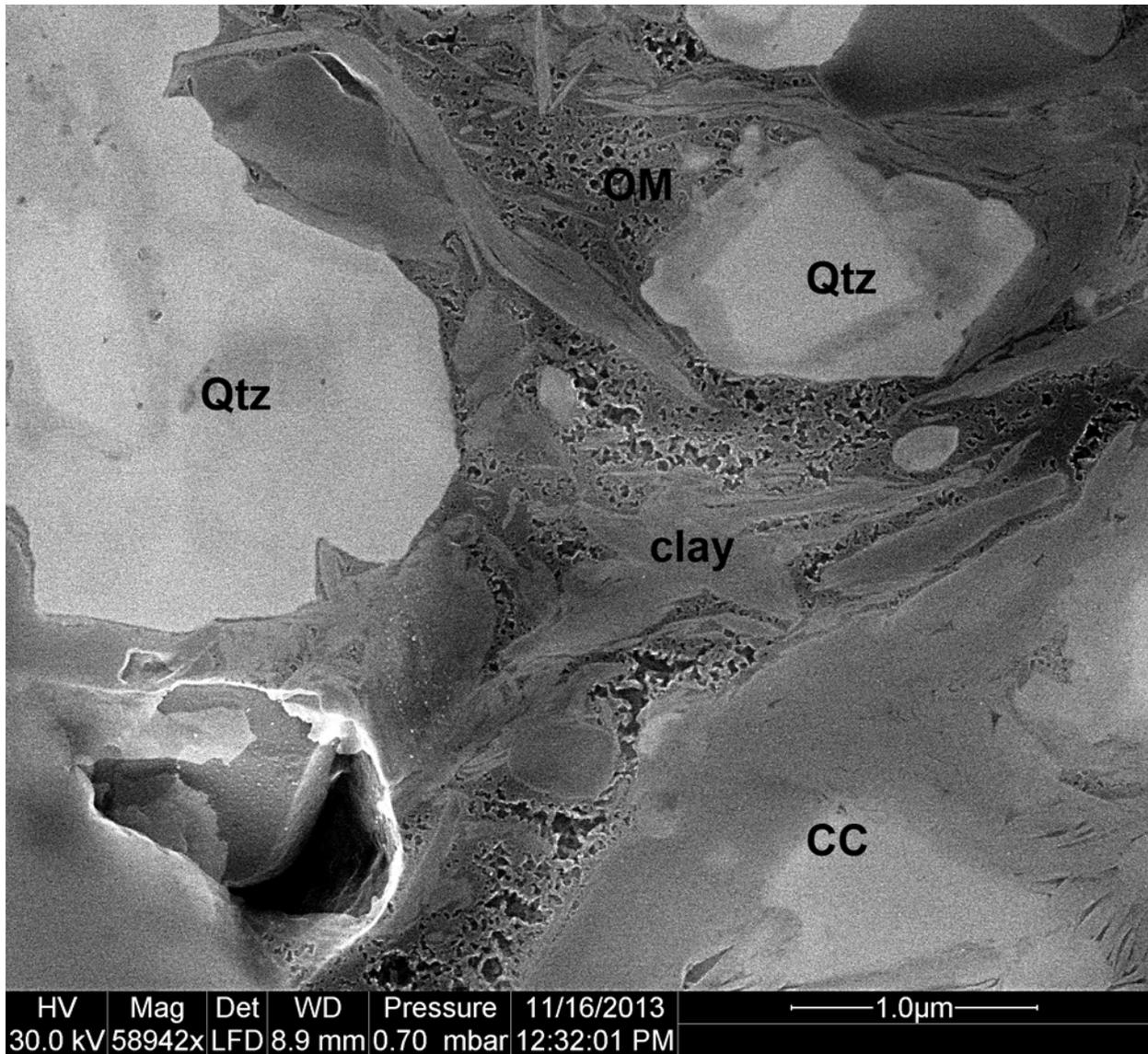
Figure 4: Another typical shale fabric close-up. Qtz=quartz, CC=calcite, OM=bitumen. With OM that shows very good OM pore development in bitumen fills and a completely open large framework pore in the lower left corner of the image.
