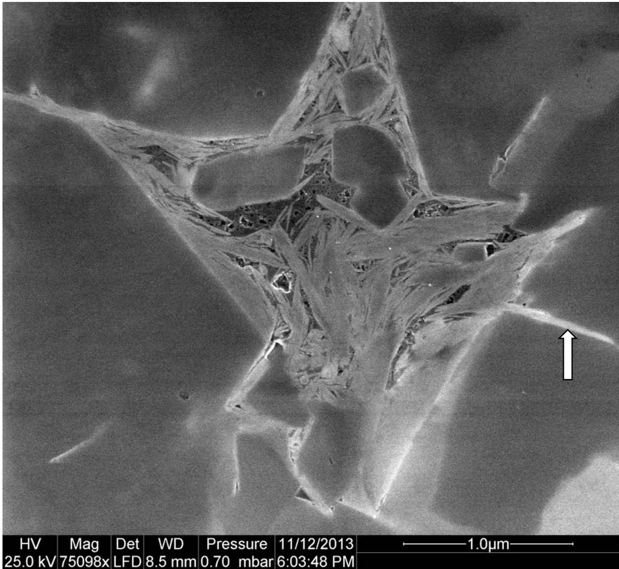
**Figure 5:** Another view of an interstitial area with a framework of clay minerals (the larger ones, >1 micron are likely detrital in origin) and an infill of organic matter between these. Later heating produced pores in the OM. Abundant early diagenetic carbonate cementation (preserves porosity by preventing compactional collapse of early pores) is indicated by the “deep” inclusion of clay platelets in carbonate/calcite grains (white arrow).
