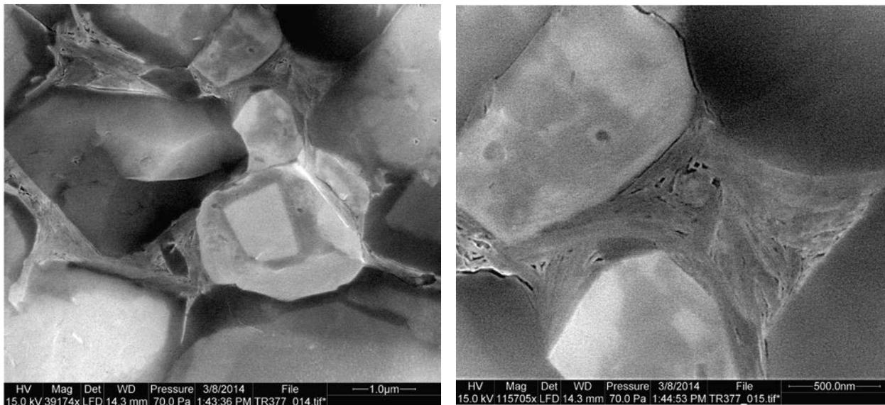
**Figure 10. Left - Pretty typical fabric with large calcite grains (dark-med gray), and in between them we have quartz (light gray) of both detrital and overgrowth nature, and a felt of clay minerals with small pores. Right - Detail of interstitial clay packing with small triangular phyllosilicate framework pores. This type of porosity probably supplies the bulk of porosity in the examined chips.**
