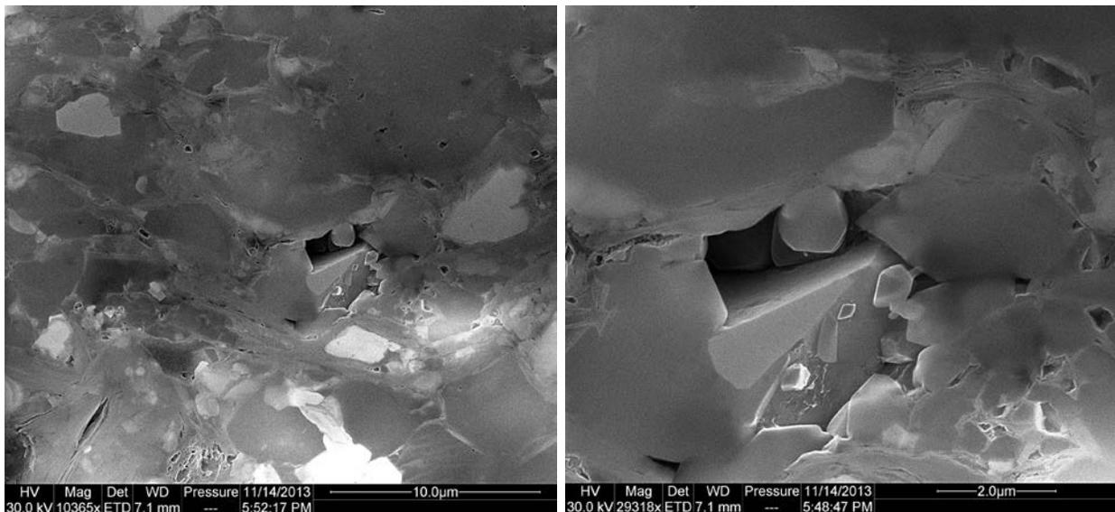
**Figure 3:** But there are in addition framework pores preserved through the support of surrounding calcite and quartz grains. The left image shows one such pore in the center, and the right image shows a close-up. In the close-up, the framework support comes largely from calcite grains, but lighter gray quartz (charge contrast imaging) is also involved.
