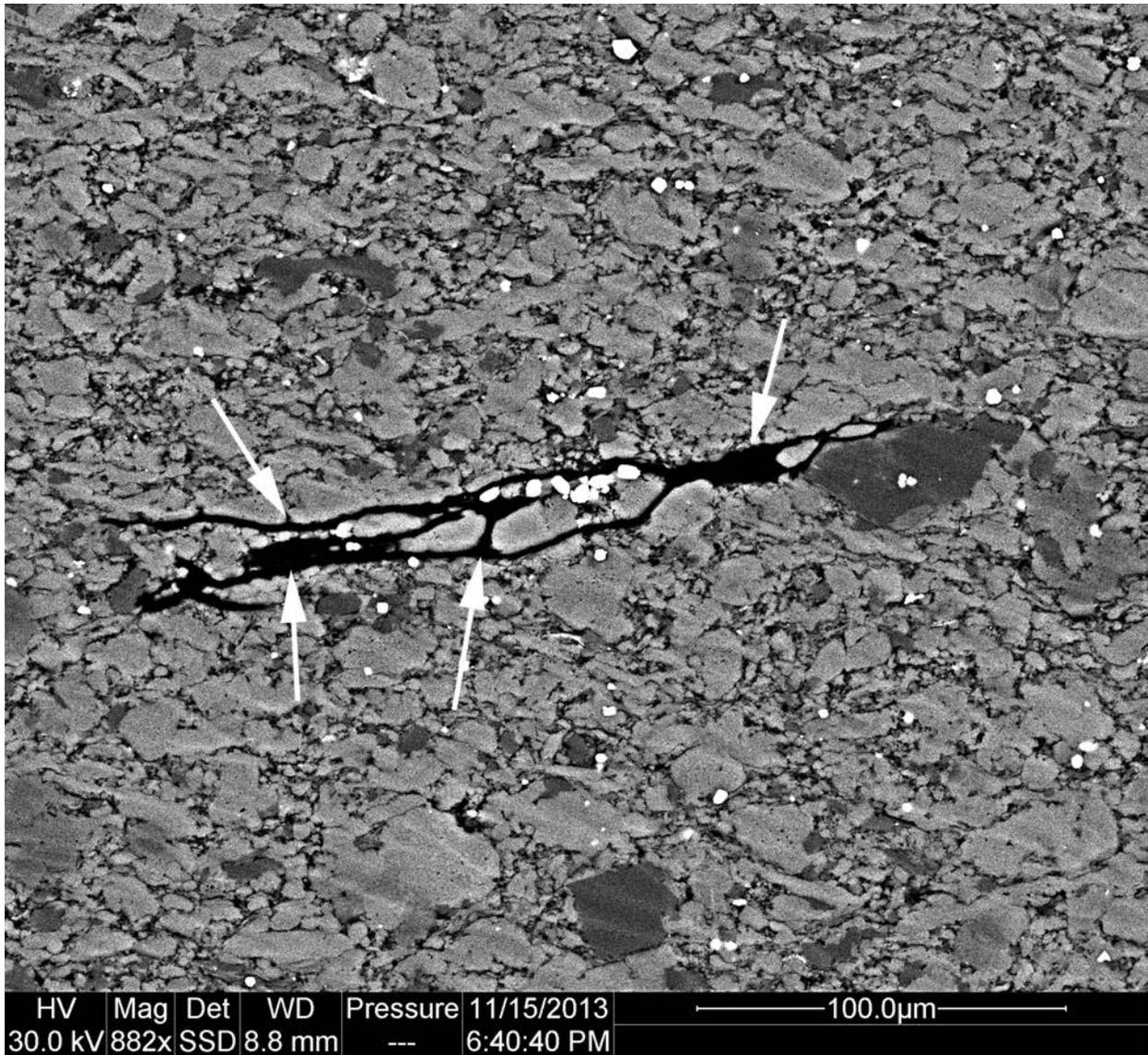
**Figure 6:** The black feature in the center of the image is a piece of organic (probably plant related) debris, and is an example of structured organic matter (cross-linked etc.). Structured OM does not show visible pores, even at high levels of thermal maturity. That latter statement applies to all samples examined.
