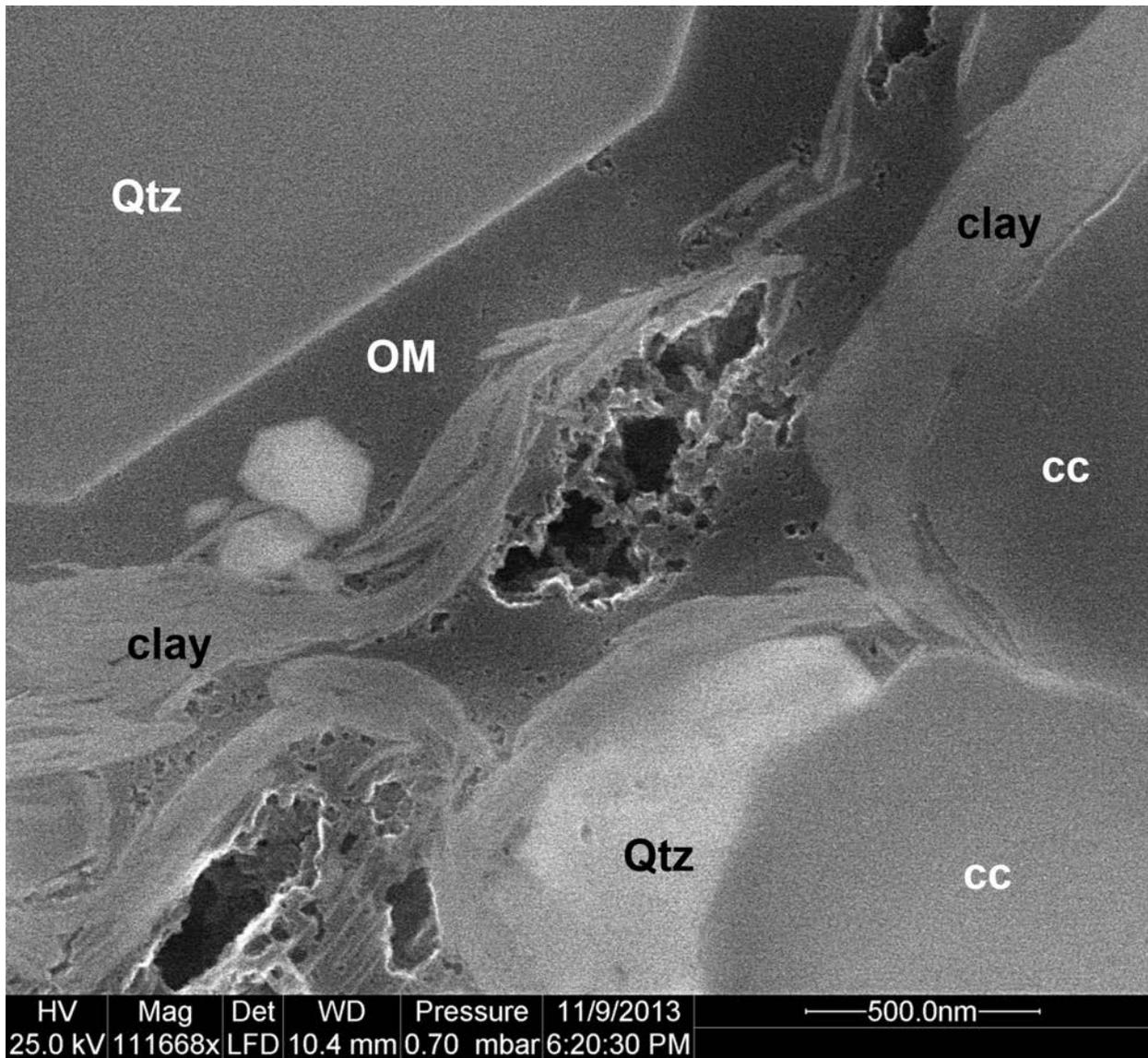
**Figure 5:** Paragenetic detail of a bitumen invaded pore space. Quartz and calcite form the primary rock fabric, and probably grew into an open pore/interstitial space (euhedral x-tal faces). Diagenetic clays formed next, and at the end the remaining pore space was filled with organic matter /bitumen. Once heated further, the bitumen “cracked”, released liquid and gaseous hydrocarbons, and pores were generated.
