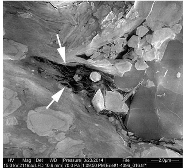
**Figure 7.** Left – Piece of likely structured OM (som) that seems to be resistant to compaction (may be some plant matter) and has strange triangular pores (not sure what that is). But it does not have pores in the matrix and is ion-beam “resistant”. Right –Typical appearance of amorphous OM (dark, arrows) with intermingled clays.
