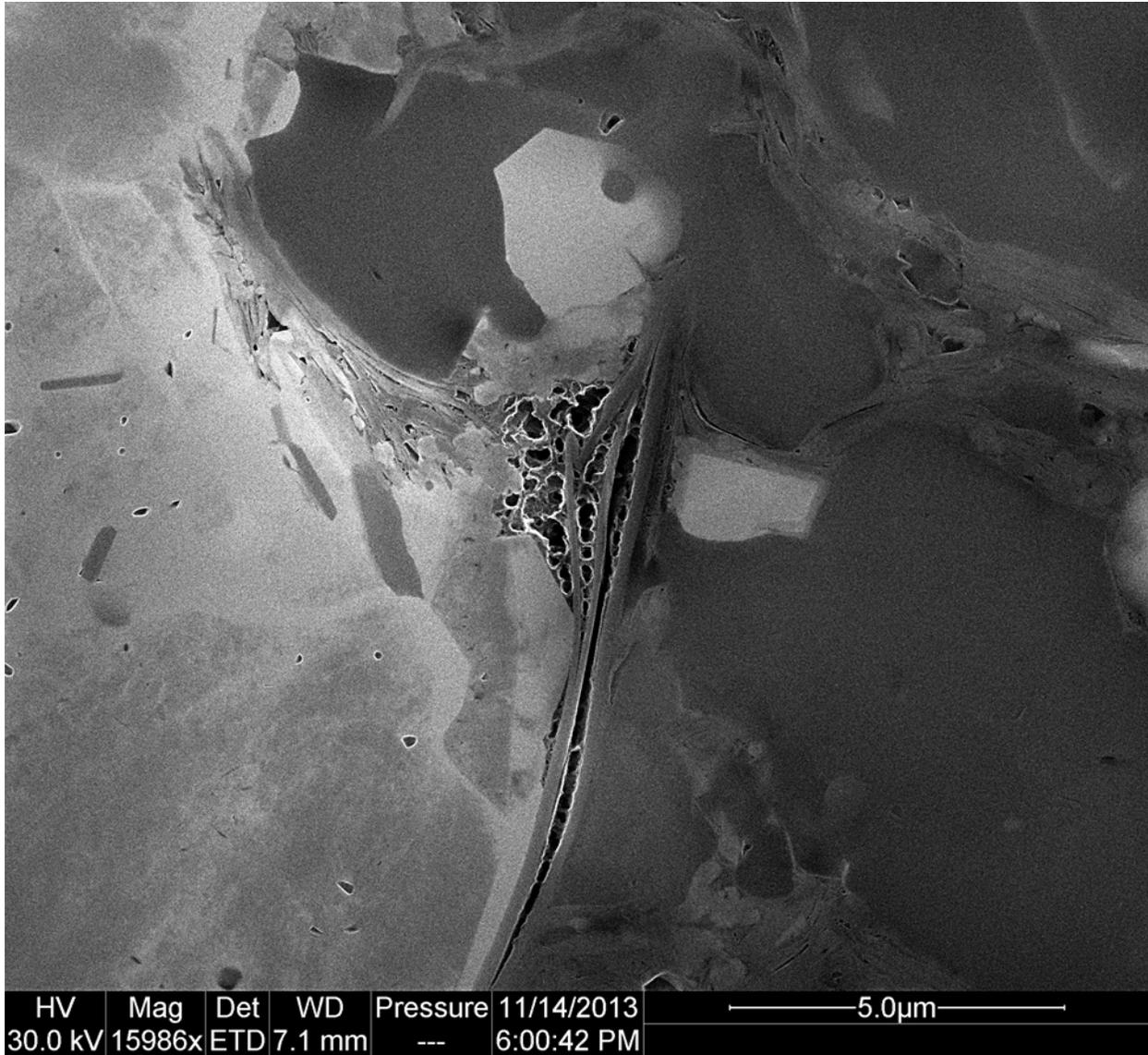
**Figure 5:** Another example of interstitial Om with very well developed OM pores. Here the OM infilled between sheets of a mica grain that splayed open in an existing pore space prior to hydrocarbon formation and infilling of the space with (likely) bitumen. The next image shows details of the OM porosity.
