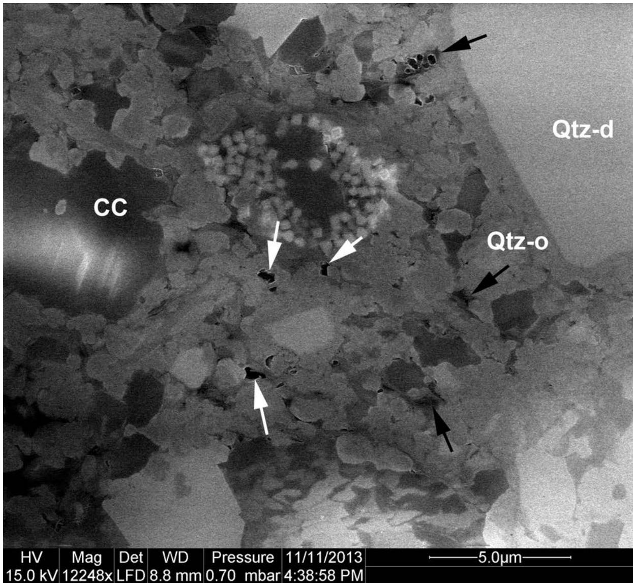
**Figure 2:** Shale fabric with abundant diagenetic quartz that supports framework pores (white arrows). In places these quartz framework pores are filled with organic matter and diagenetic clays (black arrows). Diagenetic silica varies across the sample, but the association between diagenetic silica, organic matter, and clays is pervasive. CC=calcite, Qtz-o = overgrowth and diagenetic quartz, Qtz-d = detrital quartz.
