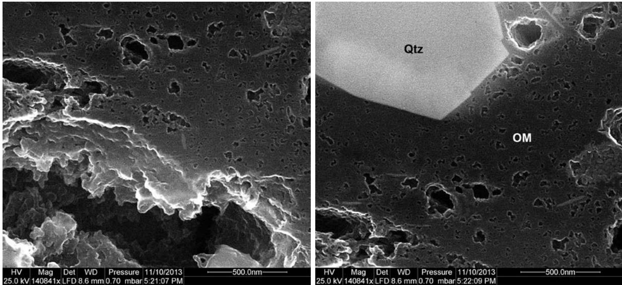
**Figure 9:** OM pore development in the bitumen fill seen in Fig. 8. Shows well developed bubble pores and abundant foam pores in the 10-50 nm size range.
