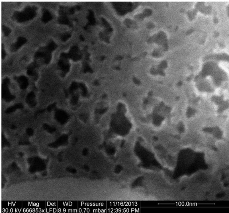
**Figure 8:** Very high magnification image of OM from Fig. 7. Pores as small as 5 nm in size can still be recognized.
