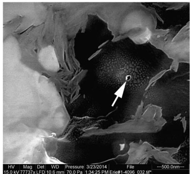
Figure 8. Left – Closer high magnification view of amorphous organic matter (OM) that is mingled with clays and diagenetic quartz (qtz). There is no porosity visible in the OM. Right – Another close-up view of amorphous OM. The ion beam burned a hole into the OM (arrow) and the surface of the OM has developed the characteristic dimpled appearance that occurs when the beam is vaporizing OM. This OM is probably “soft” hydrocarbons, probably bitumen.
