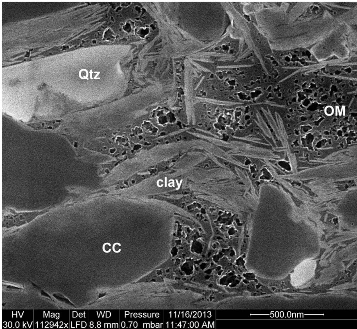
**Figure 5:** Detail view of the interstitial OM/clay assemblage. CC=calcite; Qtz=quartz. Shows well developed OM porosity with a mixture of larger bubble pores (connectivity/conduction) and smaller foam pores (storage).
