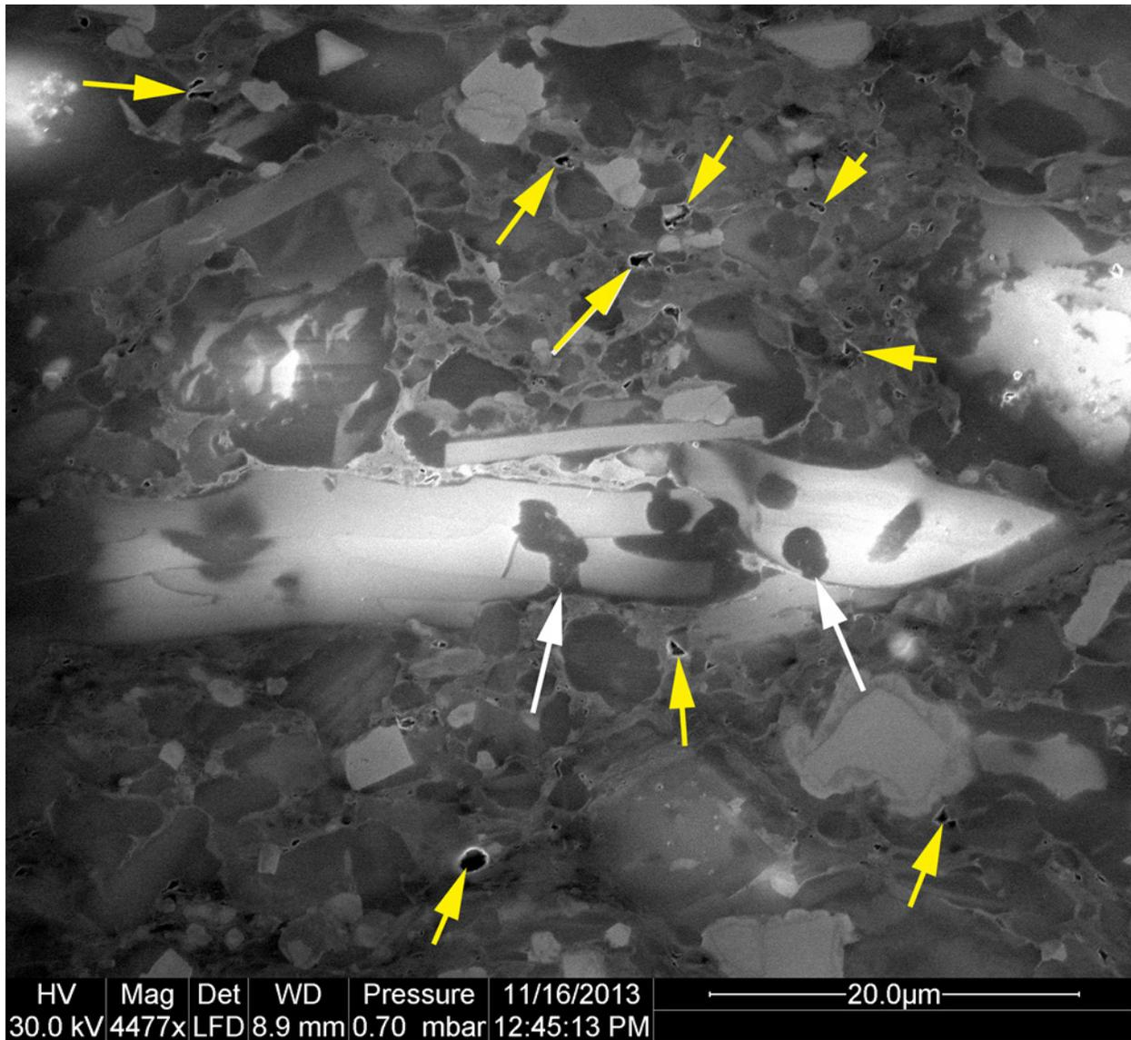
Figure 2: Overview of a (at first) pretty tight appearing shale fabric. The shell fragment in the center of the image (bright) consists of calcite, and has borings filled with dolomite (darker gray, white arrows; formed very early in diagenesis). The yellow arrows point to open framework pores (calcite and quartz defined). In addition, many interstitial spaces between larger mineral grains contain pore filling bitumen that has developed OM-pores.
