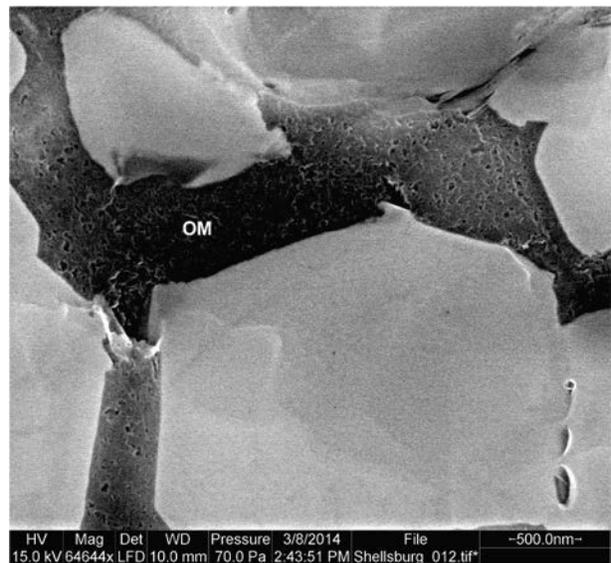
**Figure 2. Left – Close-up of interstitial space with abundant phyllosilicate framework pores. This pore type is rather common in these chips. Right – Large pores in carbonate grain. They look like pores that are continuing into depth, and may be remains of carbonate framework pores (with the carbonate having recrystallized). These pores are comparatively rare.**
