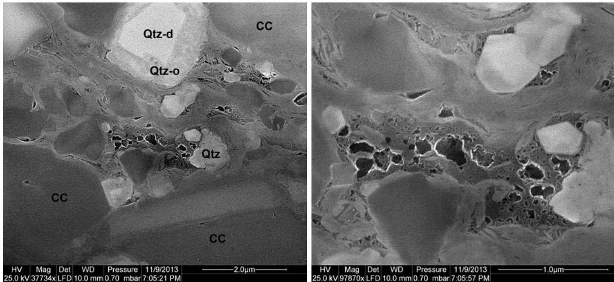
**Figure 5:** Anotehr nice example of interstitial organic matter with good development of OM pores (foam and bubble). And in left image clear development of abundant diagenetic overgrowth quartz (Qtz-o) on detrital quartz. Qtz=quartz, CC=calcite.
