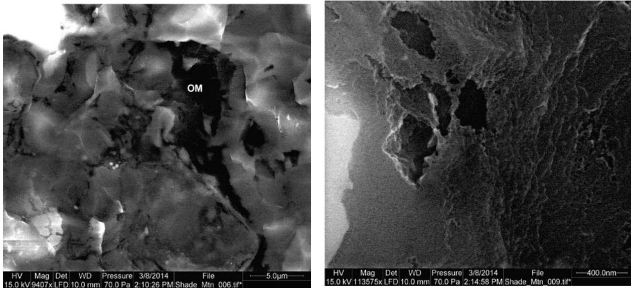
**Figure 9. Left – Interstitial OM within the overall tight fabric of these chips. Right – Detail of interstitial OM, showing tiny foam pores in the OM matrix, and large “bubble” pores in the 100’s of nm size range. These formed probably as a consequence of liquid hydrocarbon migrating out of this source rock.**
