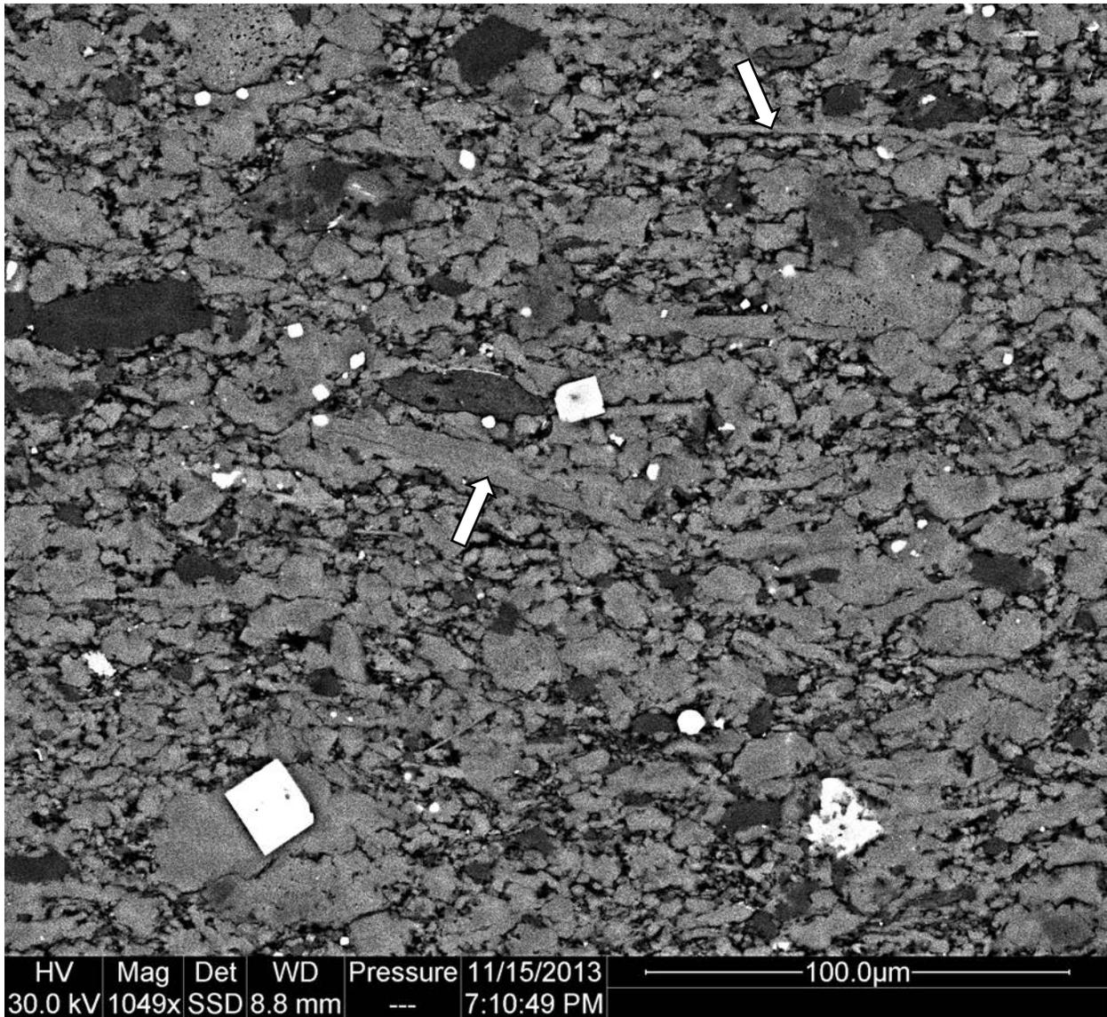
Figure 2: Shale fabric at higher magnification (backscatter image). The dominant color is light gray, due to calcite (this field of view suggests dominance of carbonate over terrigenous components). The dark grey blebs in the tens of micron size range are quartz grains, the clay minerals and organic matter are squeezed in the interstitial areas between larger mineral grains. White arrows point to fragments of thin fossil shells. Most likely thin shelled benthos. Very bright grains are pyrite.
