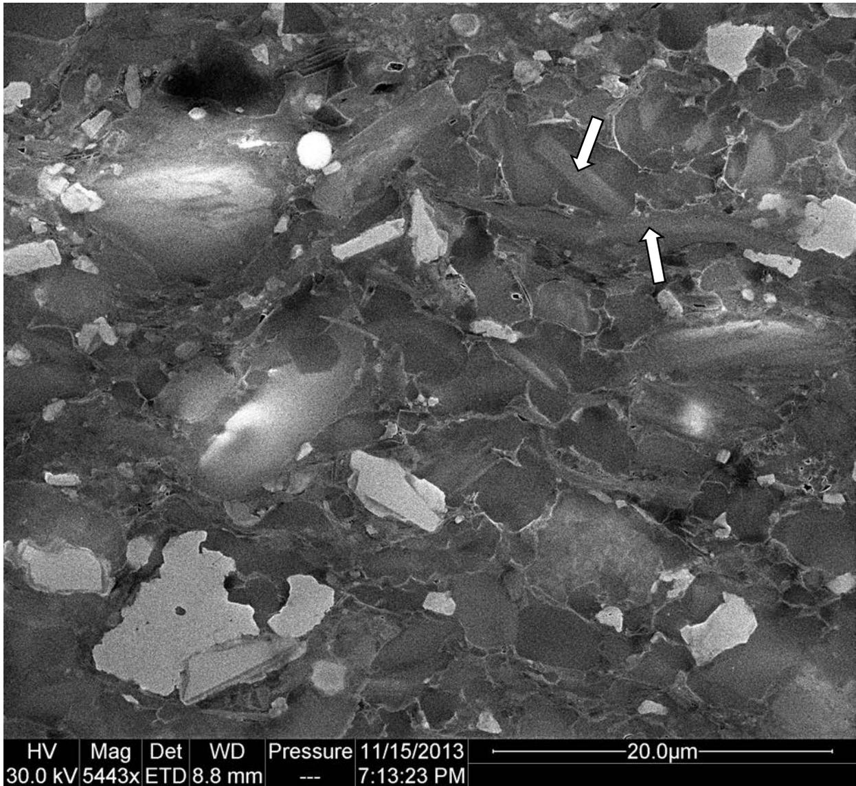
**Figure 3:** Shale fabric at even higher magnification (SEM mode, charge contrast image). The light gray grains are quartz (detrital with overgrowth, and also all diagenetic). Most of the medium to darker gray grains are carbonate/calcite. Some of these contain slightly lighter lath-shaped cores (white arrows) which are probably fossil debris with diagenetic overgrowth. So, its possible that there is more fossil debris in here than meets the eye in a standard thin section.
