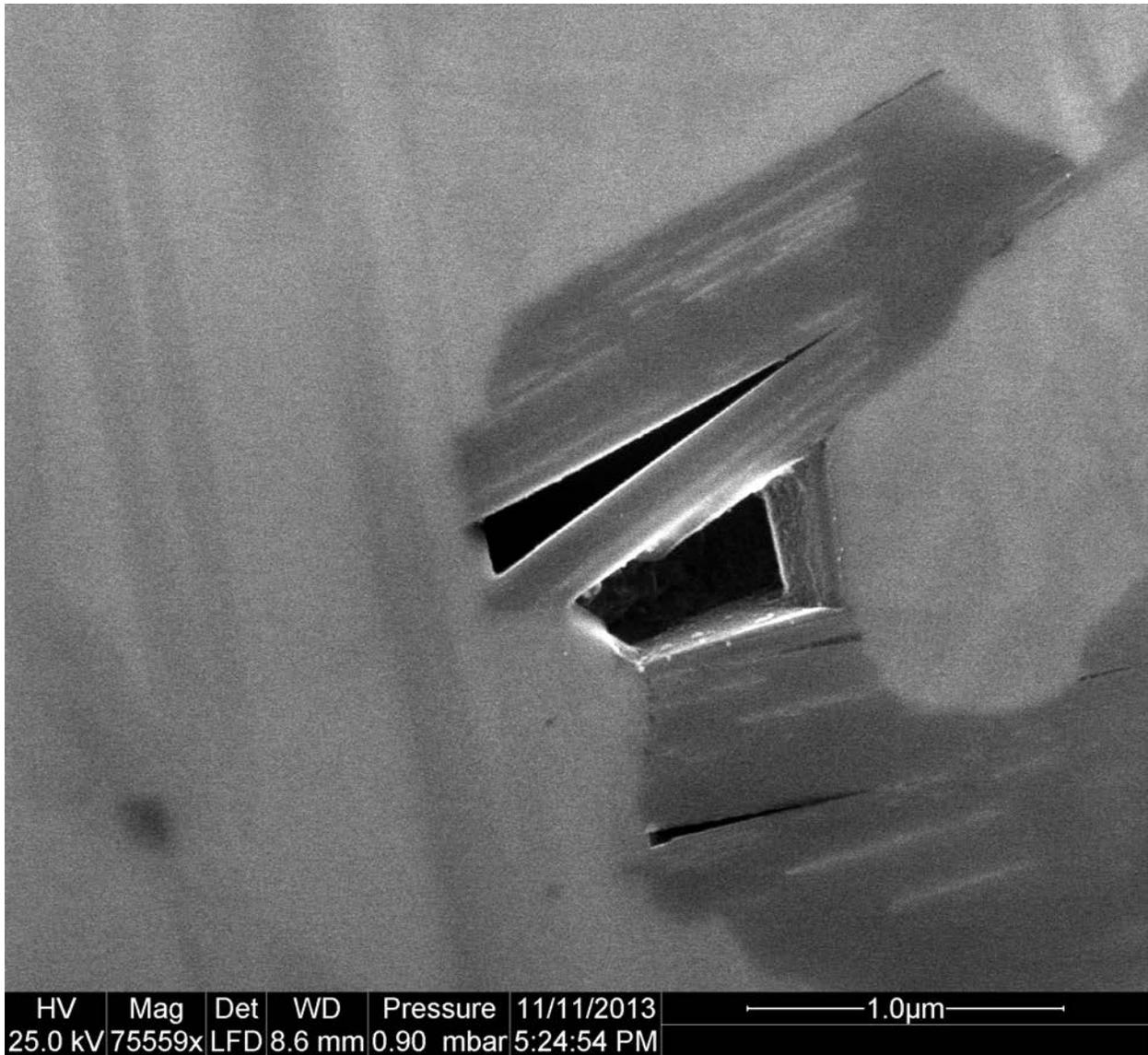
Figure 5: Example where diagenetic clay flakes have grown in a space between diagenetic quartz grains and define triangular and polygonal phyllosilicate framework pores. These are usually associated with areas of diagenetic silica cementation.
