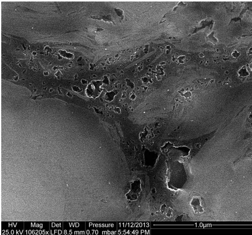
Figure 4: Close-up of OM pores from Fig. 3. The larger bubble pores are bright rimmed because of charging in low vacuum imaging mode. This the same mode of OM and OM-pore occurrence as in all previous samples (170-566 feet).
