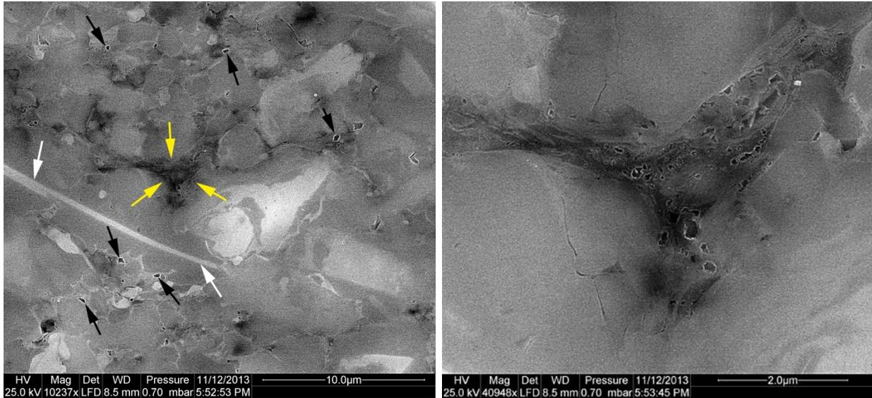
Figure 3: Closer view of shale fabric. Left image: White arrows point to calcite shell fragment. Black arrows point to open framework pores between calcite grains and (in places) quartz grains. However, due to the comparatively high carbonate content, the calcite defined framework pores dominate. The yellow arrows point to an interstitial area with abundant organic matter. Right image: Close-up of this organic-rich area. Visible are the larger bubble pores within the OM.
