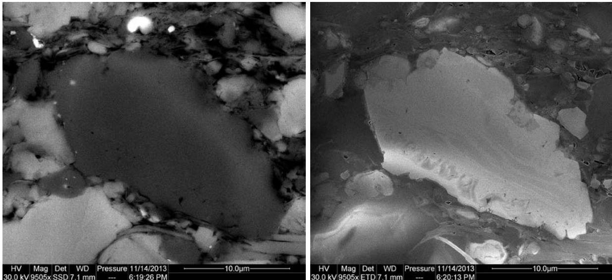
**Figure 2:** The shale matrix in close-up. At left BSE image that shows a dark gray quartz grain in the center, surrounded by light gray calcite grains, and a mixture of smaller particles that are mingled with organic matter (black). At right a secondary image in charge contrast mode that shows that the quartz grain has substantial diagenetic overgrowth, and that the dark-black areas from the left image show visible pores. These are typically in interstitial areas filled with bitumen.
