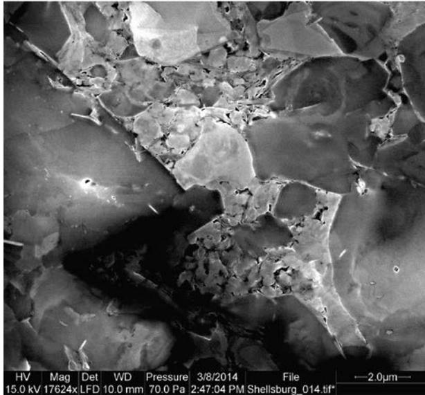
**Figure 1. Typical view of shale fabric. Larger calcite grains (dark gray) with interstitial quartz (light gray) and clays (light to medium gray, felted appearance, with triangular phyllosilicate framework pores).**
