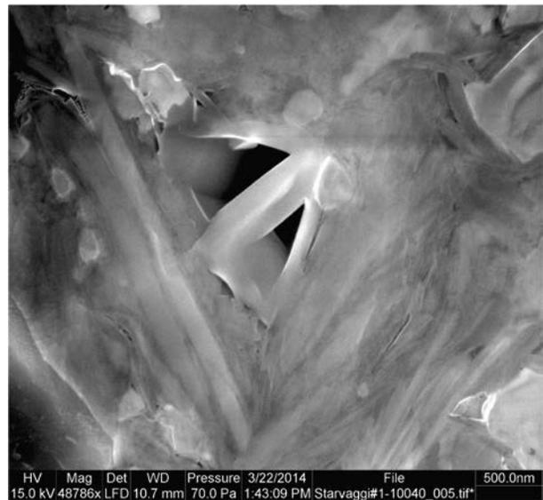
**Figure 15. Examples of phyllosilicate framework pores can be seen in these chips. Left – Clay flakes have been “clamped” by diagenetic mineral growth. Right – Clay flakes make up a support framework with triangular pores.**
