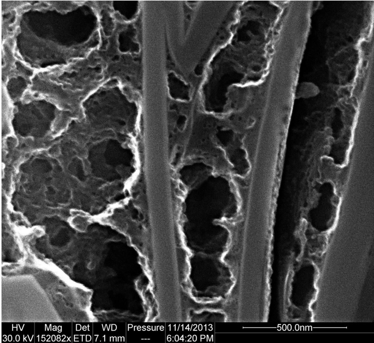
Figure 6: Detail from Fig. 5. Subvertical sheets of mica are separated by highly porous OM, probably pyrobitumen. The pores show pore throats and pore connectivity at depth.
