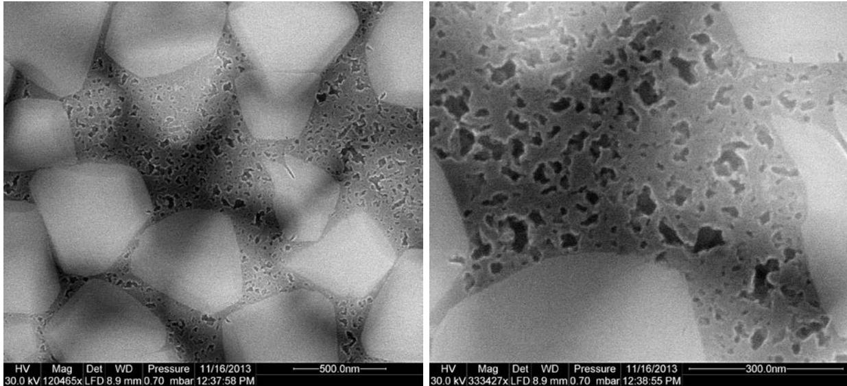
**Figure 7:** The space between the sub-crystallites of pyrite framboids very typically is infilled with kerogen (left) and that kerogen (bitumen?) also shows well developed OM pores (right). Not a significant component in the overall pore picture, but it contributes.
