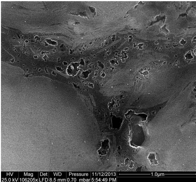
Figure 4: Close-up of OM pores from Fig. 3. The larger bubble pores are bright rimmed because of charging in low vacuum imaging mode. This is the same mode of OM and OM-pore occurrence as in all previous samples (170-566 feet).
