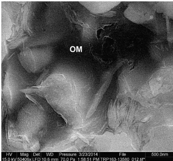
**Figure 13. Another area with interstitial OM. In this sample, larger OM pores (bubble pores) are better developed.**
