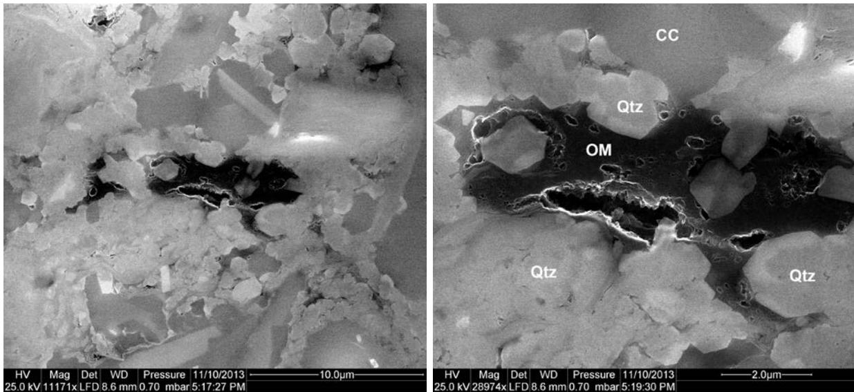
**Figure 8:** OM pore fill (dark-gray to black, in center) in the context of the overall fabric. Low mag at left, high mag at right that shows the well developed OM pores in the bitumen fill. These pores, protected from collapse by diagenetic silica cement, were most likely the travel routes of hydrocarbons when this rock produced oil.
