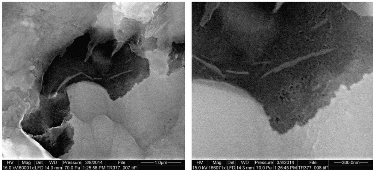
**Figure 11. Left – Pocket of interstitial amorphous OM (dark gray – black) with inclusions of clay minerals. Right – Close-up of OM that shows small pores of the “foam” type. This sample probably could have been anywhere between Ro 0.7 and 0.9.**
