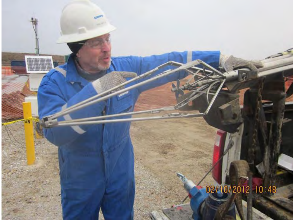
Figure 7-18. Four-arm caged full-bore spinner-logging tool.
