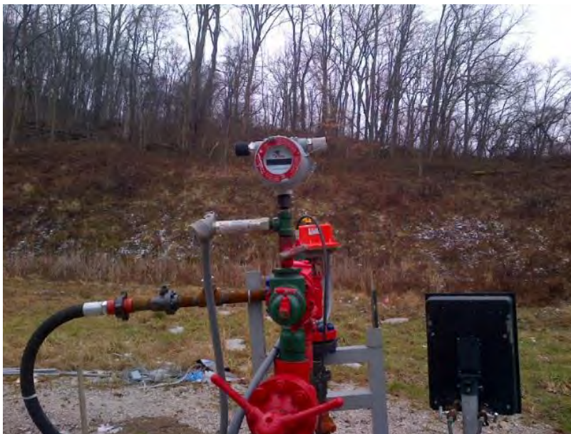
Figure 2-13. Wellhead logger installed on Class II injection well for field monitoring.
