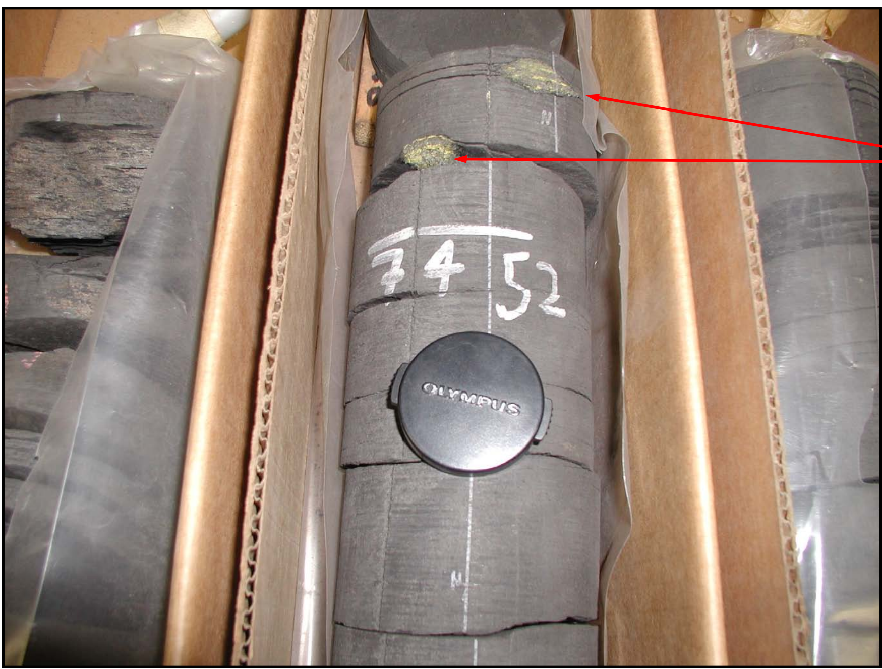
Mon 370 core, showing pyrite nodules. Lens cap is 4 cm wide.
