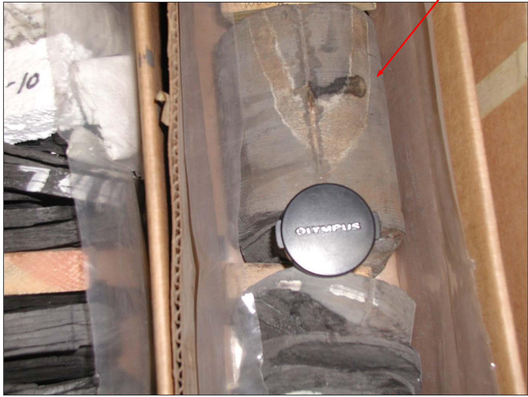
Mon 370 core showing calcareous concretion. Lens cap is 4 cm wide.
