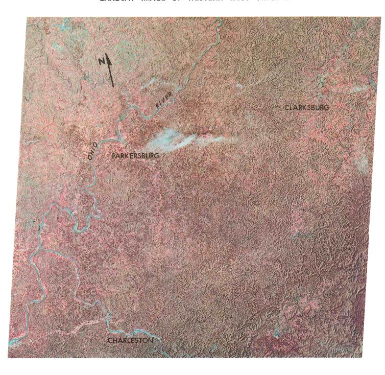
This color-infrared image was taken from the Landsat-2 satellite orbiting 575 miles above the earth. Each side of the image is approximately 100 miles long and the entire scene covers about 10,000 square miles. The satellite's sensors record reflected colors from the earth's surface in electronic form. This information is relayed to ground stations where computers are used to produce photographic-like images.
