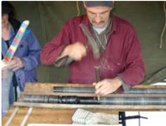
Survey geologists prepare a core from a drill site in Monongalia County.
