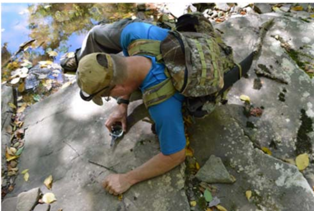
Geologist measuring strike and dip.
