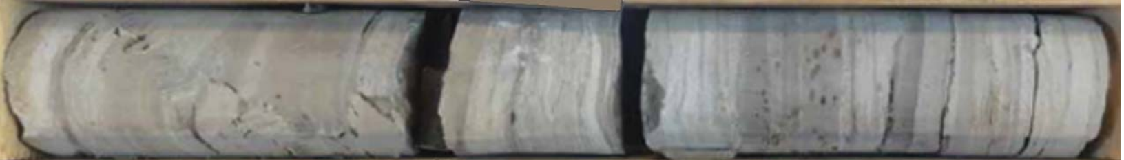
A portion of the Salina F-4 Salt core from PPG Industries Brine Well #36 (API #4705100674) in Marshall County (Photo: JP Moore)
