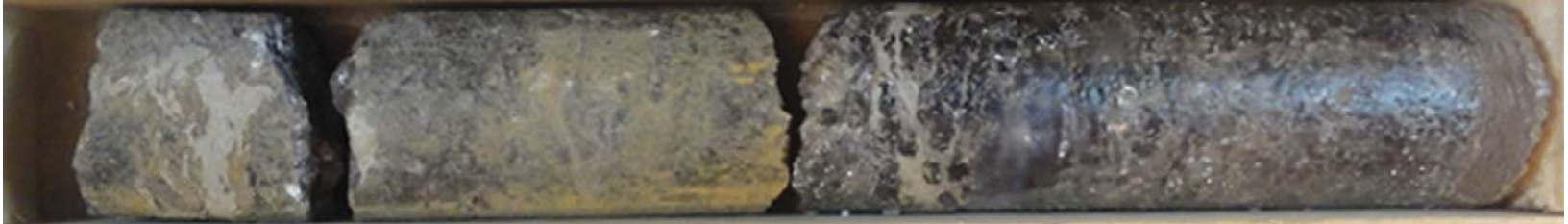
Halite in the Salina F-4 Salt core from PPG Industries Brine Well #36 (API #4705100674) in Marshall County (Photo: JP Moore)
