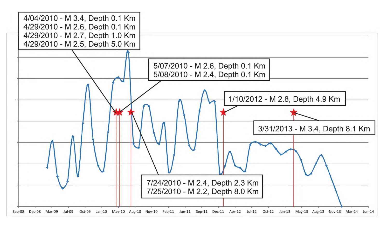
Graph of incremental injected volume vs time for well API# 4700702539. Also plotted are all Braxton County earthquakes that occurred after the well went on line in 2009. Cursory examination of this graph does not immediately indicate a connection to larger injection volumes. A time lag correspondence might be revealed by statistical analysis but if such a connection exists it must be for an extremely irregular time interval
