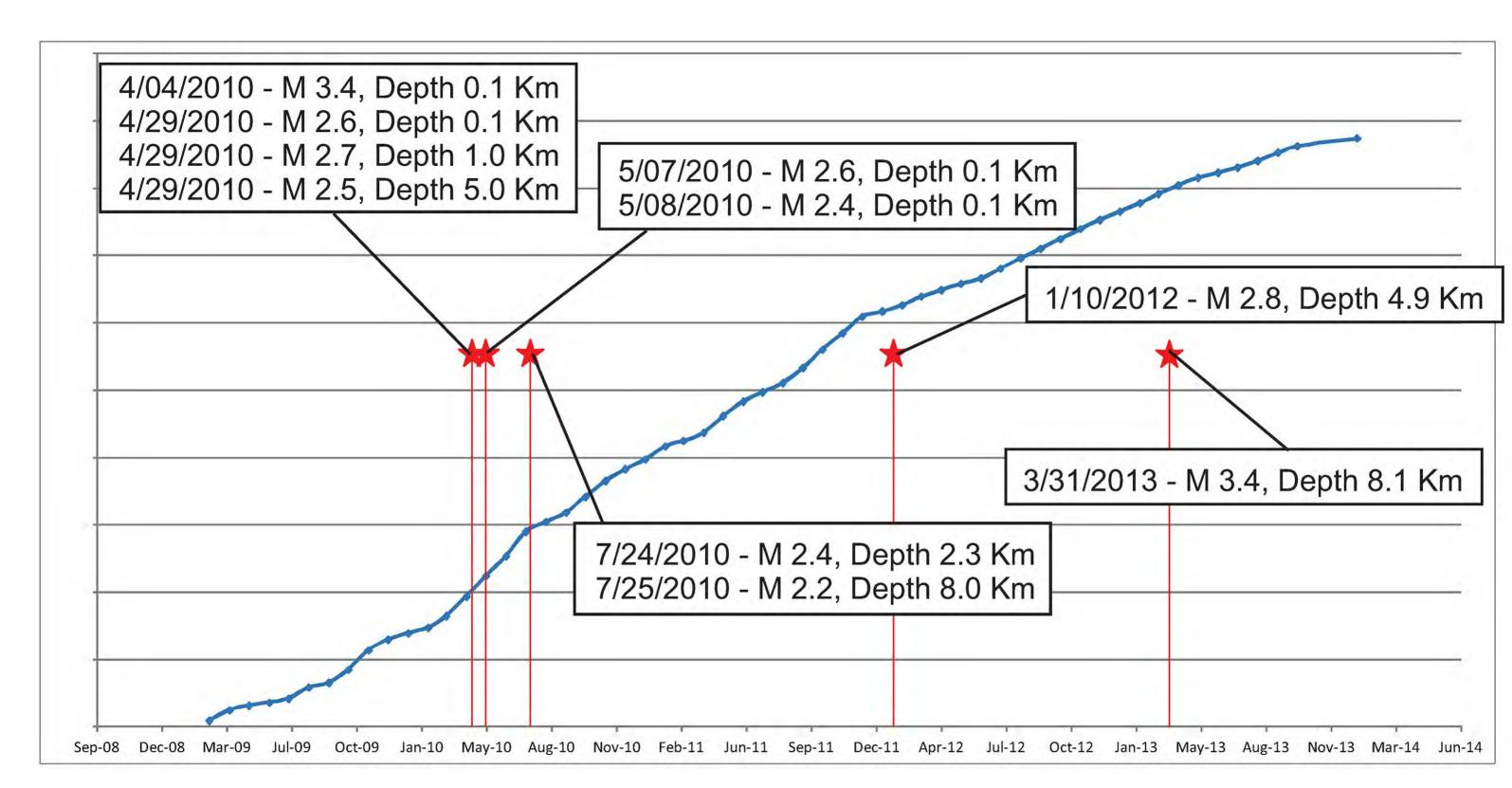
Graph of cumulative injection volume vs time for well API# 4700702539. Also plotted are all Braxton County earthquakes that occurred after the well went on line in 2009. Investigations of seismicity induced by fluid injection suggest a time lag between injection activity and earthquake events (Kerr, 2012; National Research Council, 2012). Cursory examination of this graph does not immediately indicate this kind of connection.
