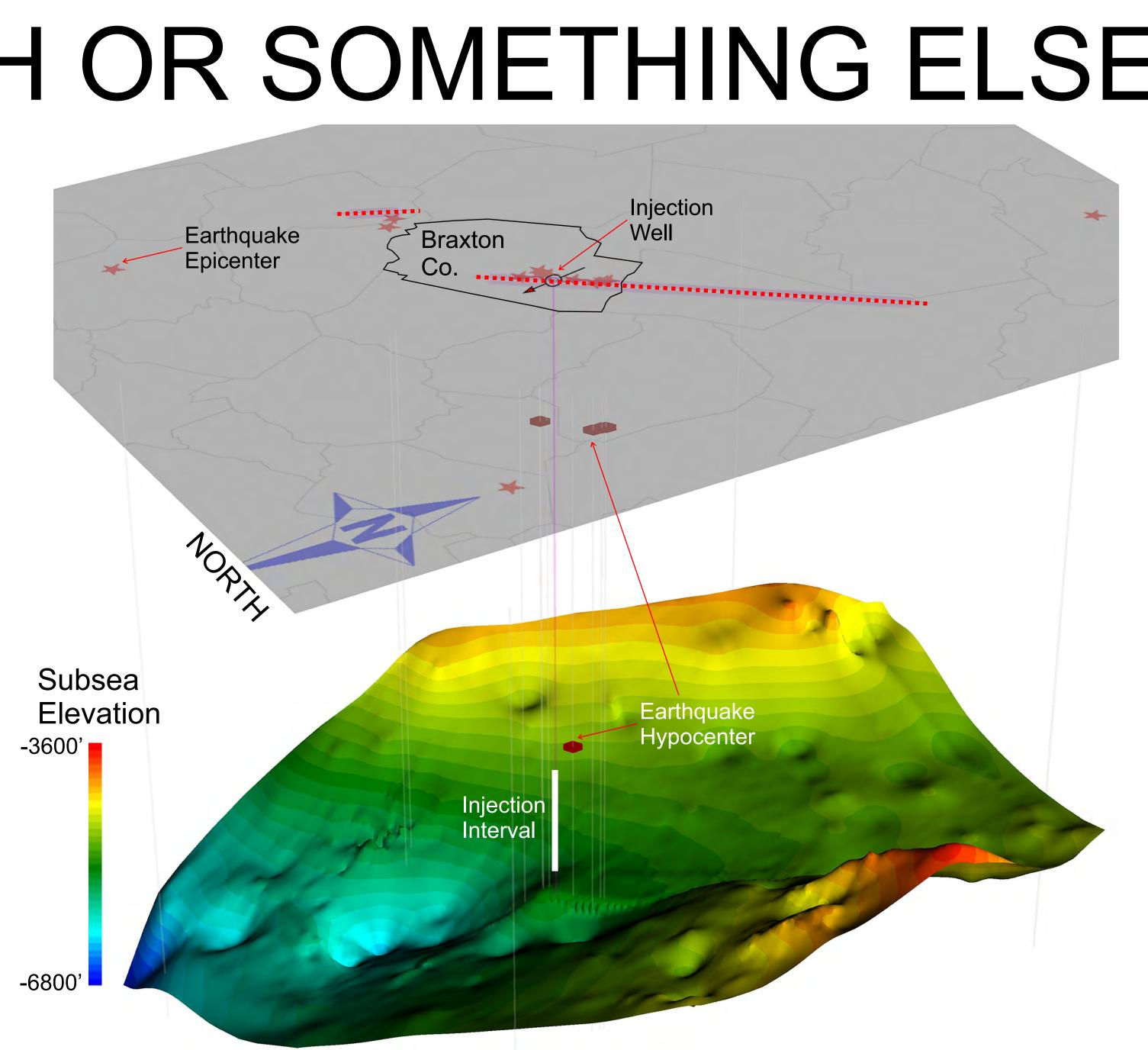
3-D modeling of the Oriskany structure in the Braxton County area indicates that the suspected fault is down-thrown to the west in the vicinity of the disposal well. Epicenters and hypocenters for earthquakes in and around Braxton County are shown as is the targeted injection interval for disposal well API# 4700705239. Vertical exaggeration is 75:1.
