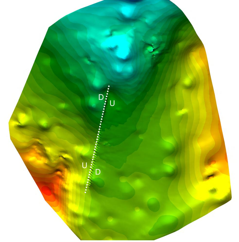
Another view of the 3-D model of the Oriskany subsea structure suggests that the suspected fault in the Braxton County area is actually a wrench fault with west side down at its north end and east side down at the south end of the fault.
